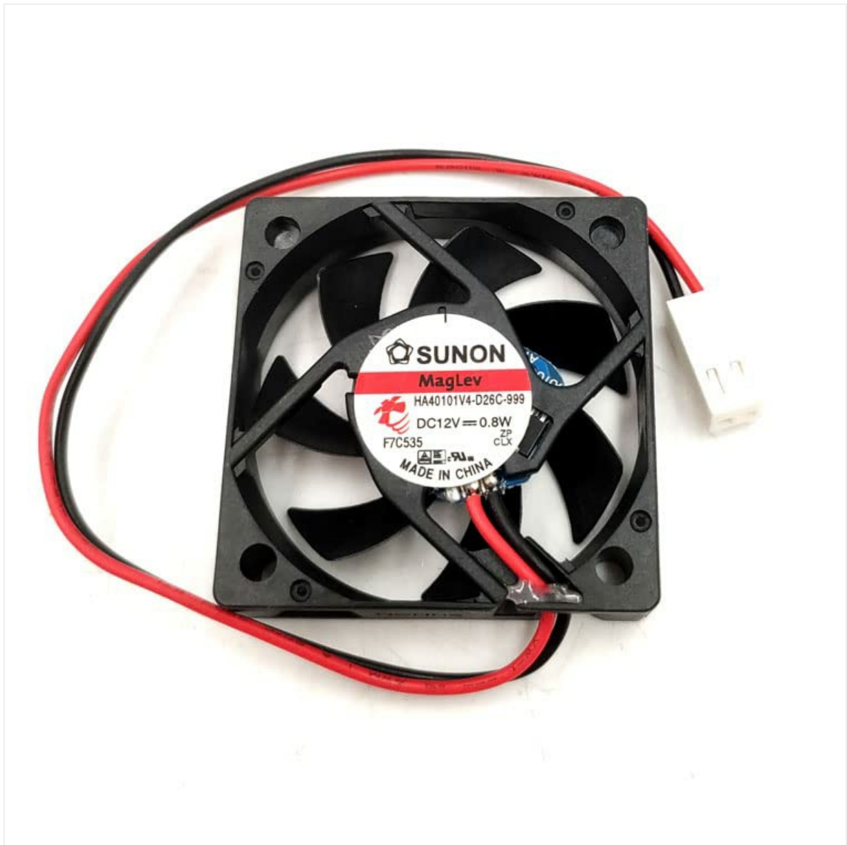
Image 1: The ELOMILE HA40101V4-D26C-999 40mm cooling fan, showing its black frame, blades, and the red and black wires leading to a white 3-pin connector. This image illustrates the fan's physical appearance and its power connection interface.
