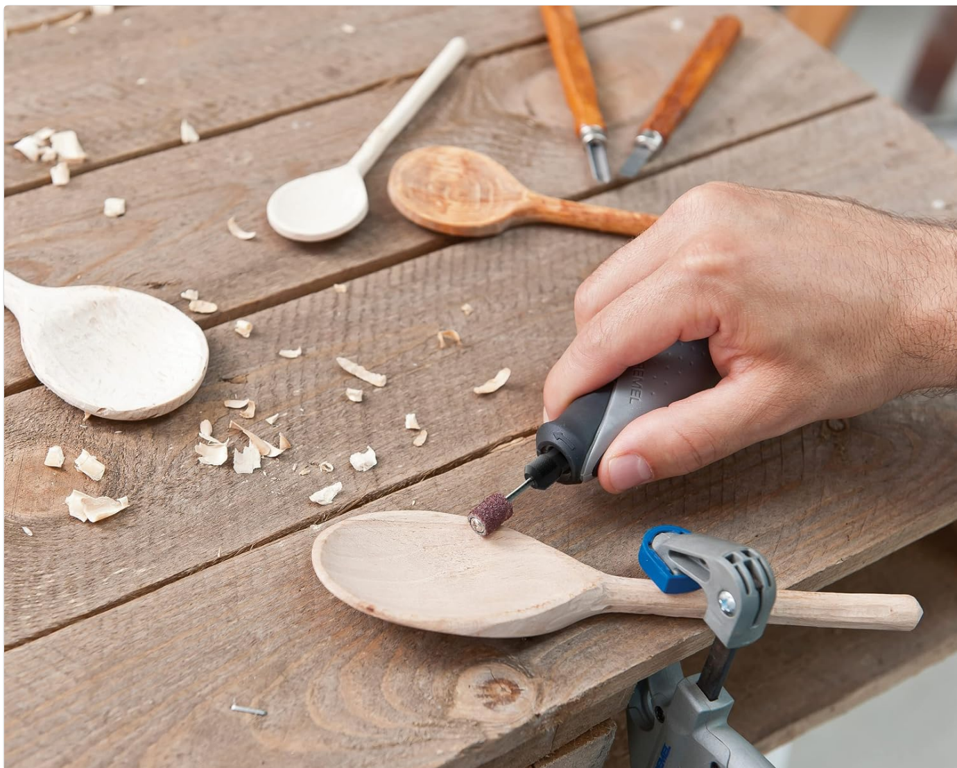
Image: A close-up of a person using the Dremel Stylo+ with a sanding accessory to smooth the surface of a wooden spoon, showcasing its utility for woodworking detail.
