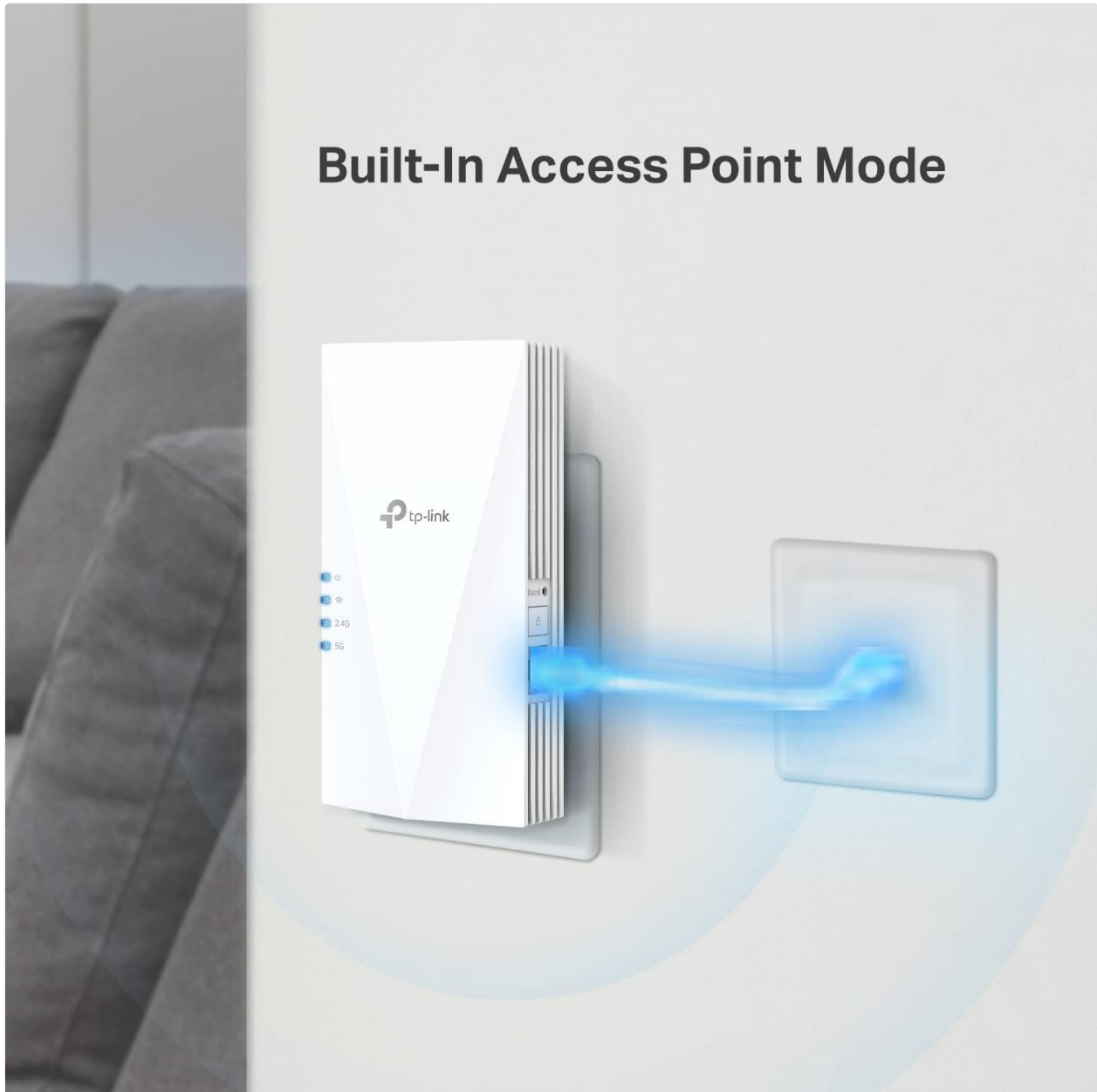
Figure 5: The RE700X operating in Built-In Access Point Mode, converting a wired connection to Wi-Fi.
