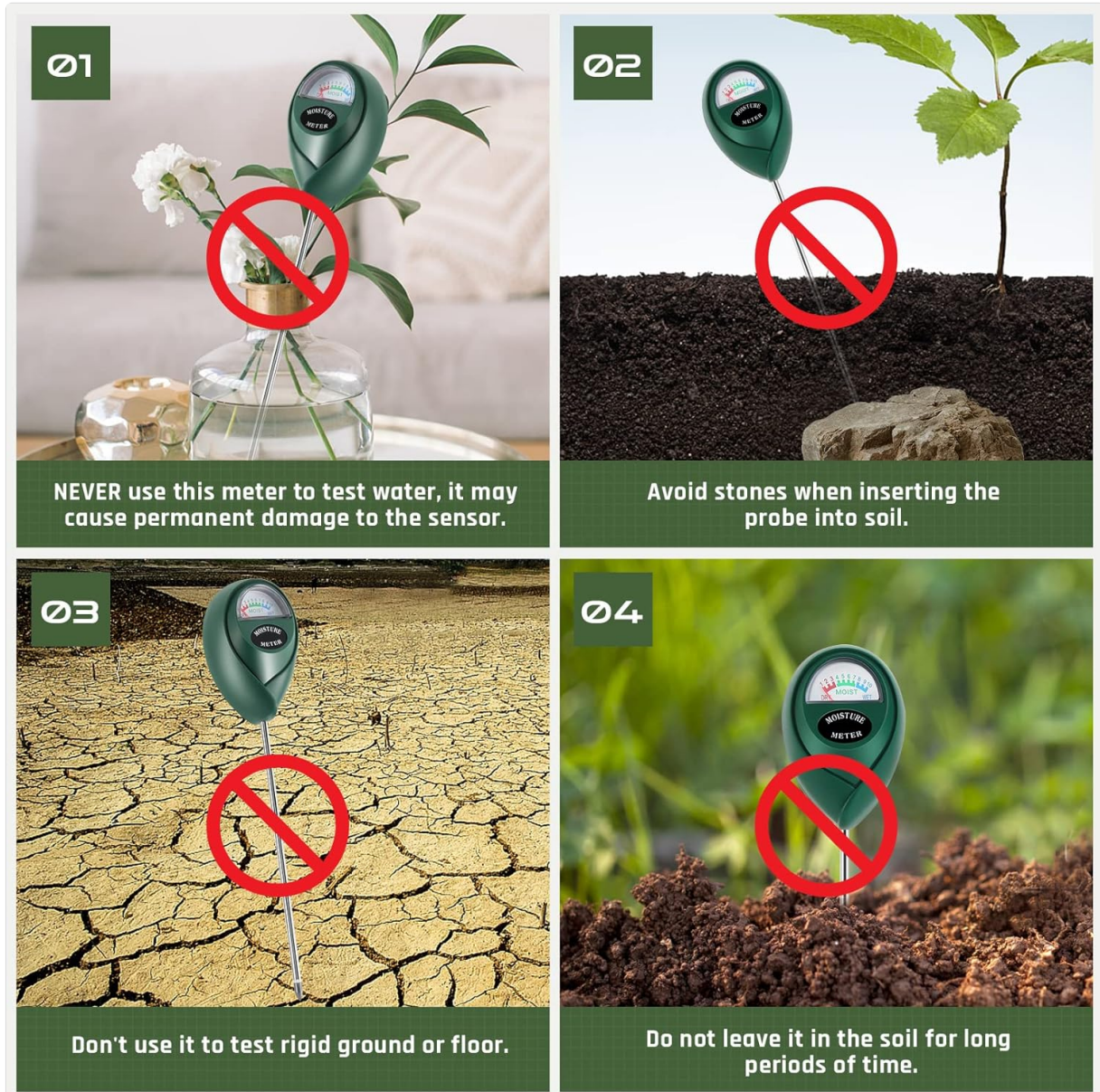
Figure 5: Visual warnings illustrating improper uses of the soil moisture meter that can lead to damage or inaccurate readings.
