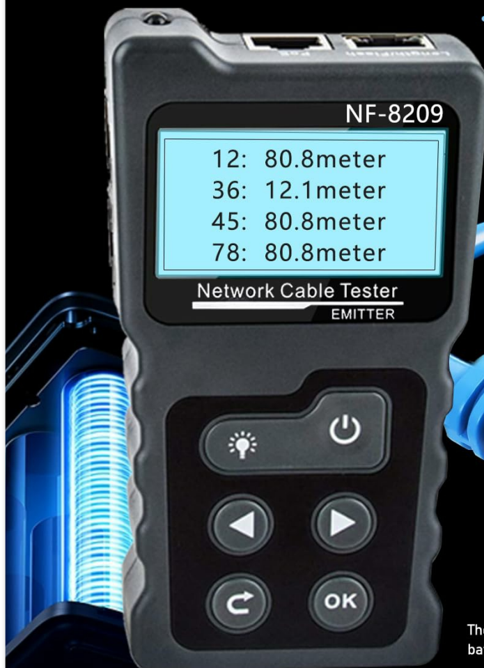
Figure 3: Cable length measurement in progress on the NF-8209 Emitter.
