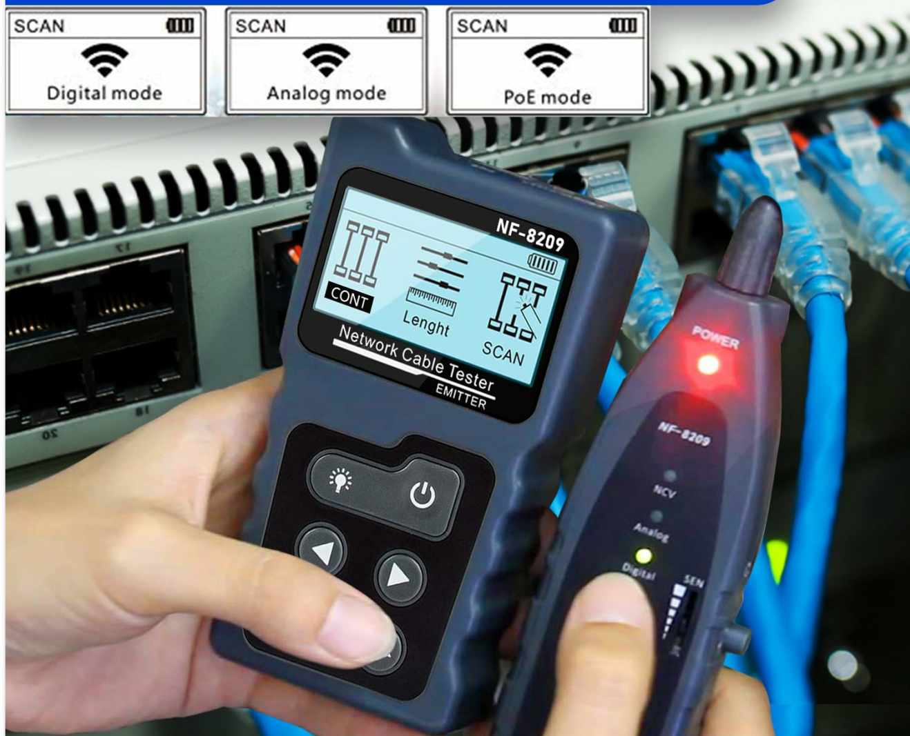
Figure 4: Selecting a tone trace mode on the NF-8209 Emitter.
