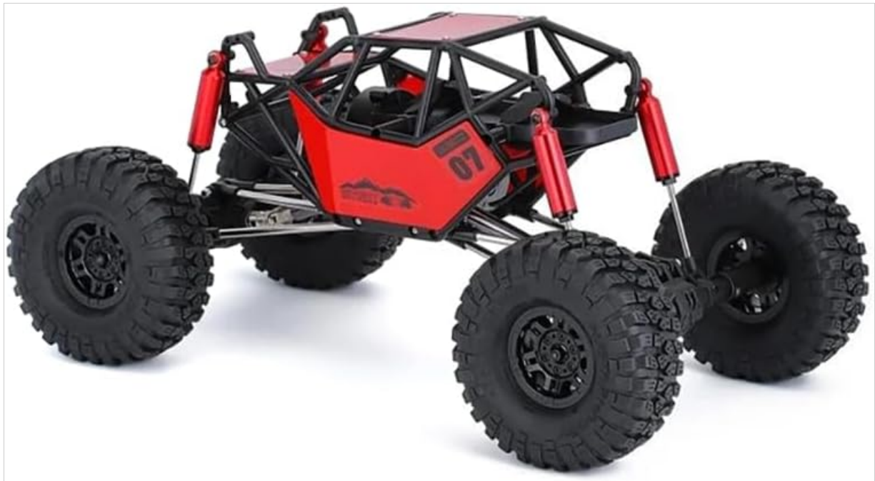
Figure 3.2: Side-front view of the chassis kit, highlighting the suspension and wheel assembly.
