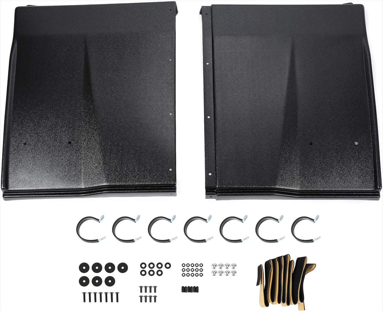
Image 3.1: All included components for the HECASA Hard Roof Top.
