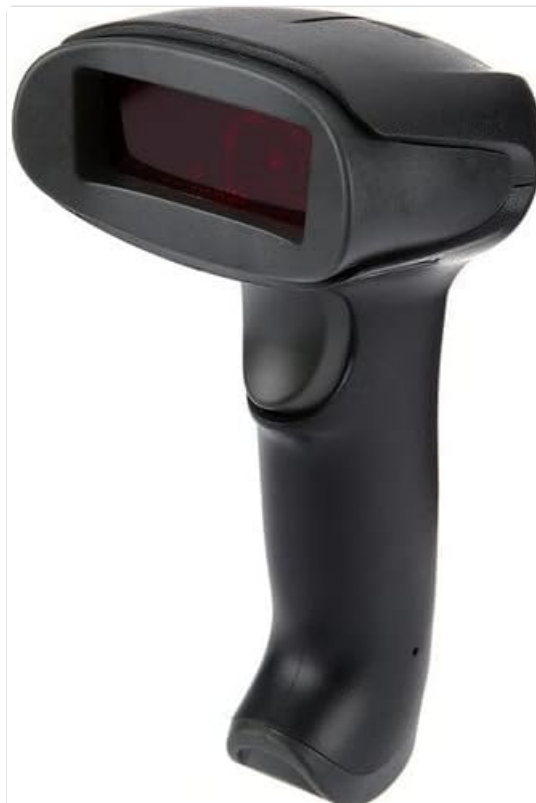
Figure 4.2: Front view of the Netum NT-2028 barcode scanner, highlighting the scanning window and ergonomic grip.
