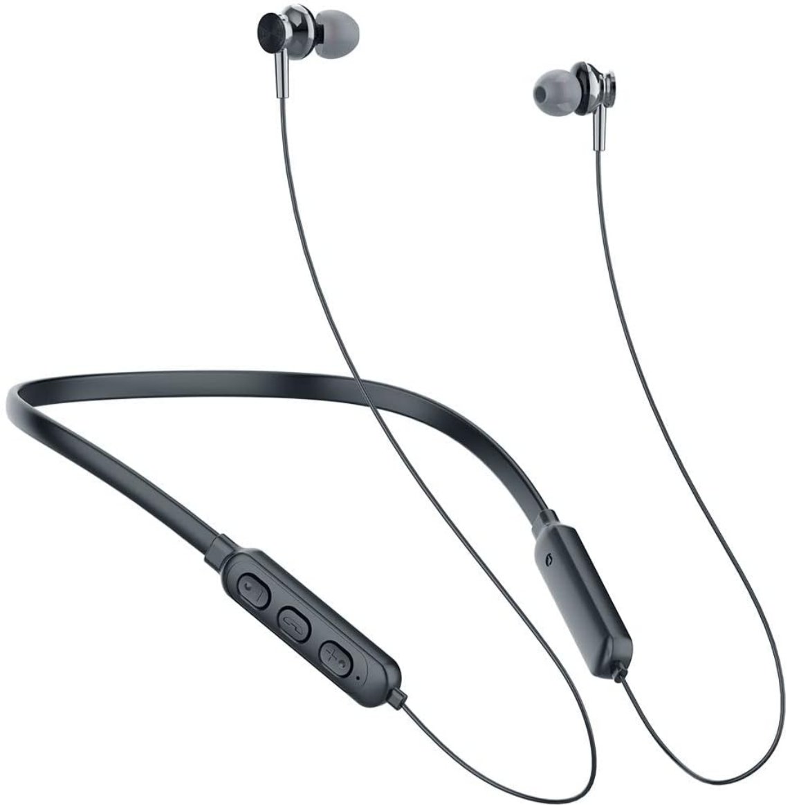
Figure 3.1: Front view of the VIDVIE BT859 headset, showcasing the neckband and magnetic earbuds.
