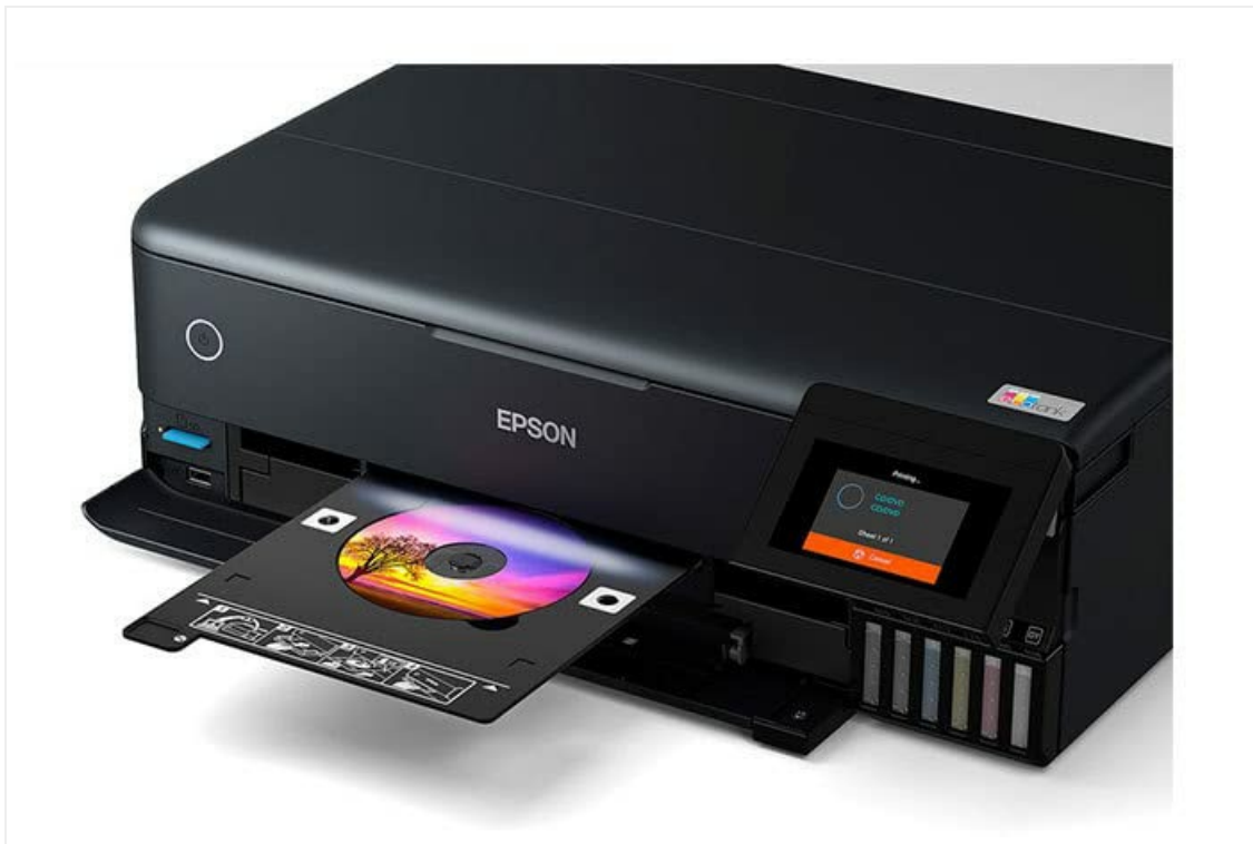
Figure 4: CD/DVD Printing Function. This image shows a printable CD being loaded into the Epson EcoTank L8180 printer's dedicated tray for direct disc printing.
