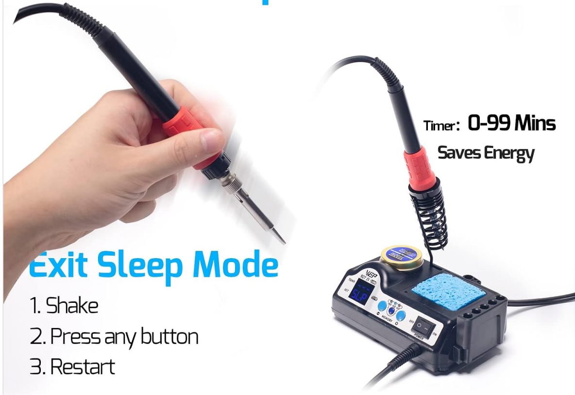
Figure 4.3: Soldering station entering and exiting sleep mode.
