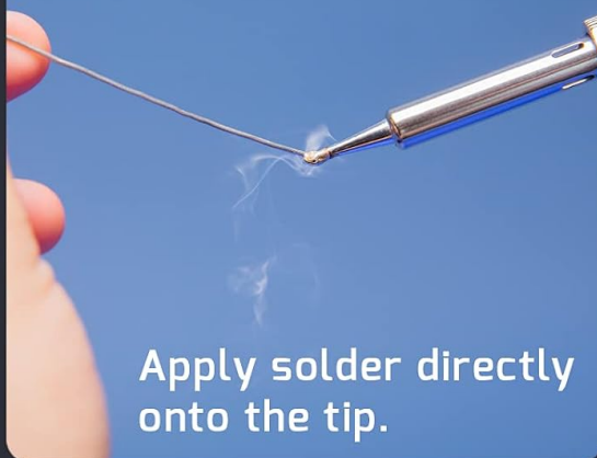
Figure 5.1: Proper maintenance and servicing of soldering iron tips.
