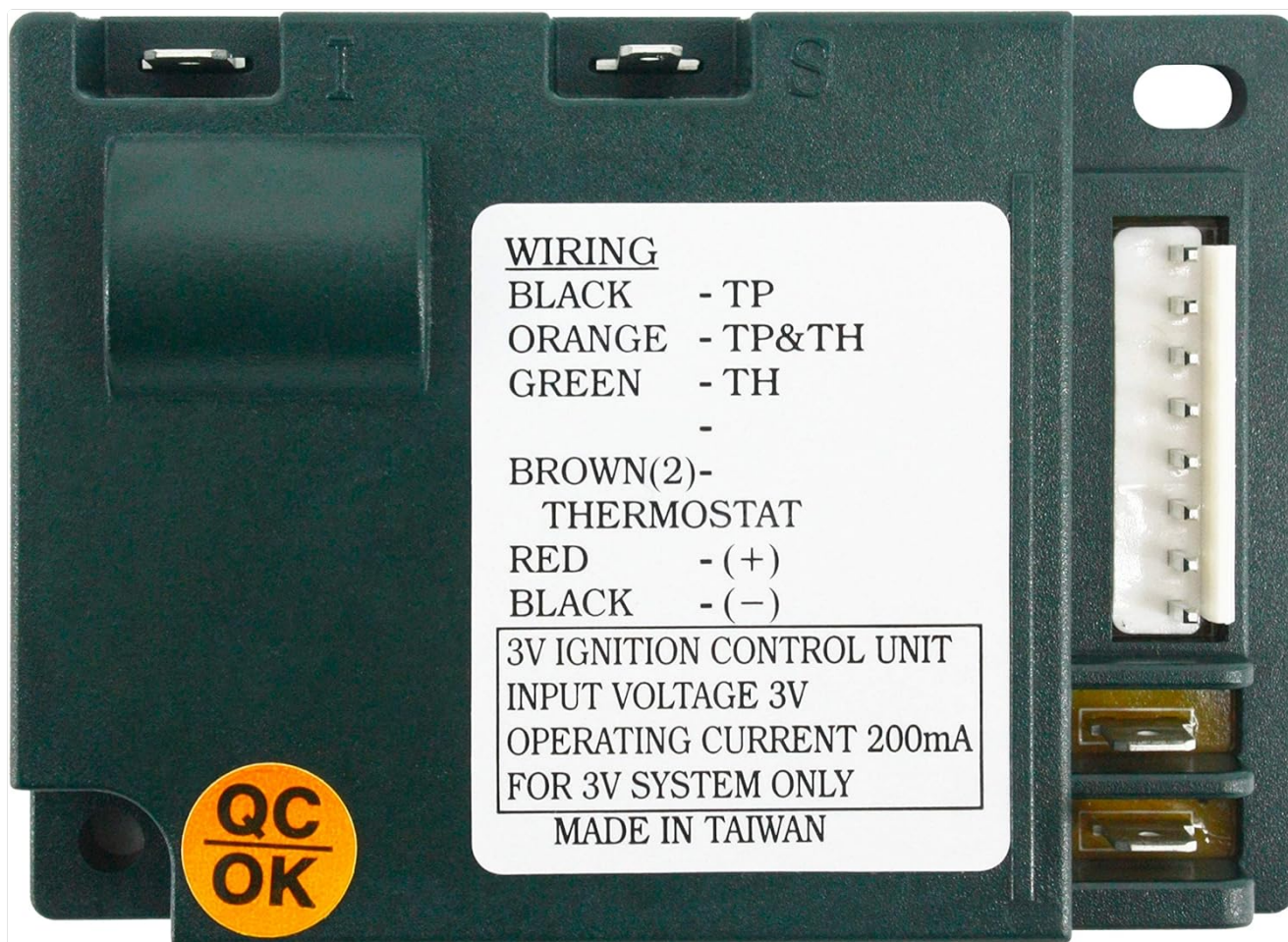
Image: Top view of the Durablow IPI-6000 Pilot Ignition Control Module. The module features a label detailing wiring connections for TP (Black), TP&TH (Orange), TH (Green), Thermostat (Brown), and battery connections (Red for positive, Black for negative). It specifies a 3V input voltage and 200mA operating current, suitable for 3V systems only, and is marked 'Made in Taiwan'.
