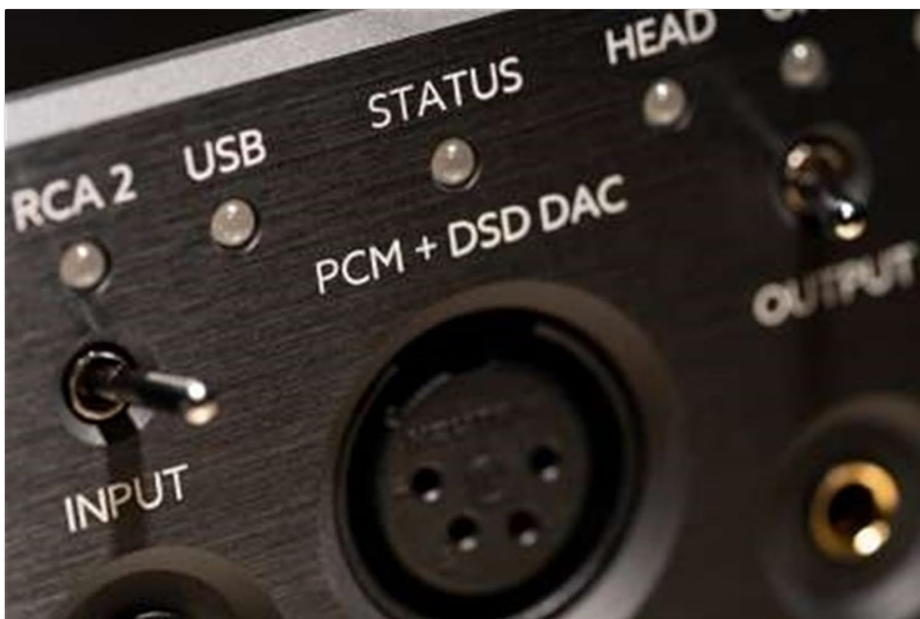
Figure 2.3: Detail of input and output selection switches.
