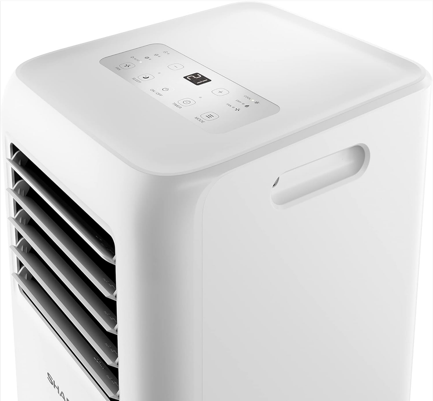
Figure 3.4: Close-up of the top control panel with LED display. The panel includes touch-sensitive buttons for power, fan speed, mode selection, timer, and temperature adjustment.
