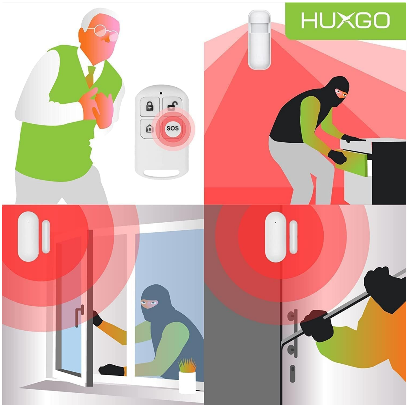
Image 5.1: Visual representation of alarm scenarios, including an intruder triggering a motion sensor or door/window sensor, and the use of the SOS button on the remote control for emergencies.
