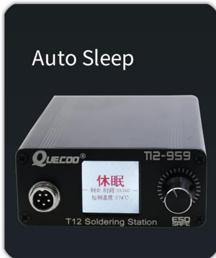
Figure 5.1: The Auto Sleep feature display on the QUECOO T12-959, showing the remaining sleep time and current temperature.
