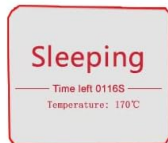
Figure 5.1: The Auto Sleep feature display on the QUECOO T12-959, showing the remaining sleep time and current temperature.
