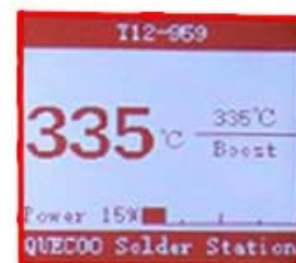
Figure 5.2: Display showing the Auto Standby feature (left) and the Boost function (right) on the QUECOO T12-959.
