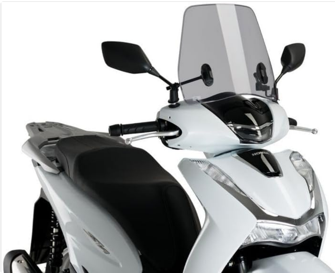
Image 3.1: A closer view of the Puig Traffic Urban Windscreen (20363H) installed on a white Honda scooter, highlighting the mounting points near the handlebars and mirrors.
