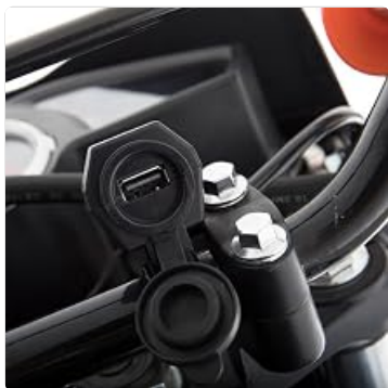
Figure 6: Integrated USB charging port located on the handlebars for convenient device charging.
