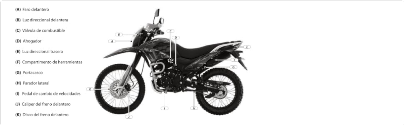
Figure 3: Labeled diagram of the ITALIKA DM250, indicating major components such as (A) Front headlight, (B) Front turn signal, (C) Fuel valve, (D) Choke, (E) Rear turn signal, (F) Tool compartment, (G) Helmet holder, (H) Side stand, (I) Gear shift pedal, (J) Front brake caliper, and (K) Front brake disc.
