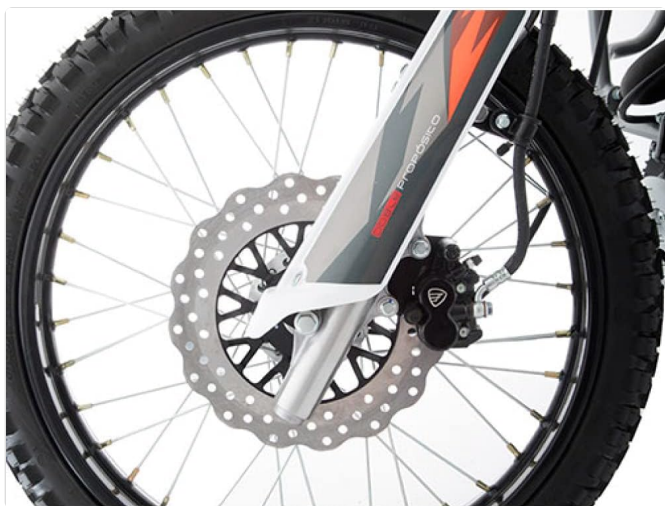
Figure 4: Detail of the front wheel and disc brake system, highlighting the robust design for reliable braking.
