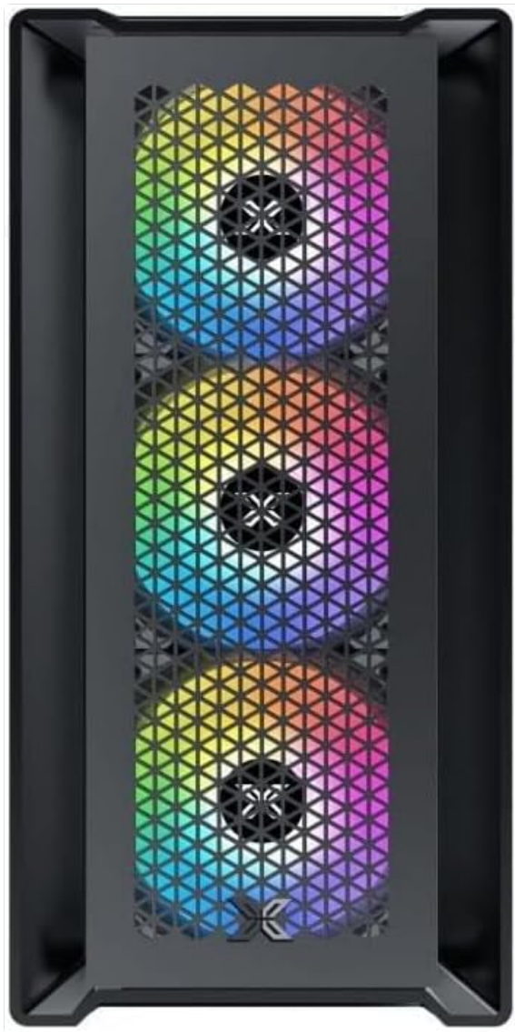
Figure 4.1: Front View. This image displays the front of the Xigmatek Lux M case, highlighting the metallic mesh panel with a triangular design and the three pre-installed 120mm fixed RGB fans.
