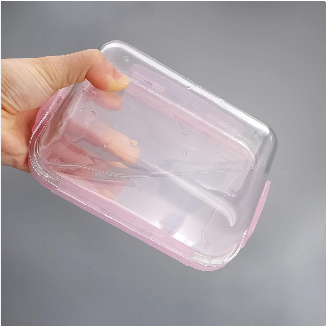
Figure 6: Testing the seal by filling the container with water and checking for leaks.
