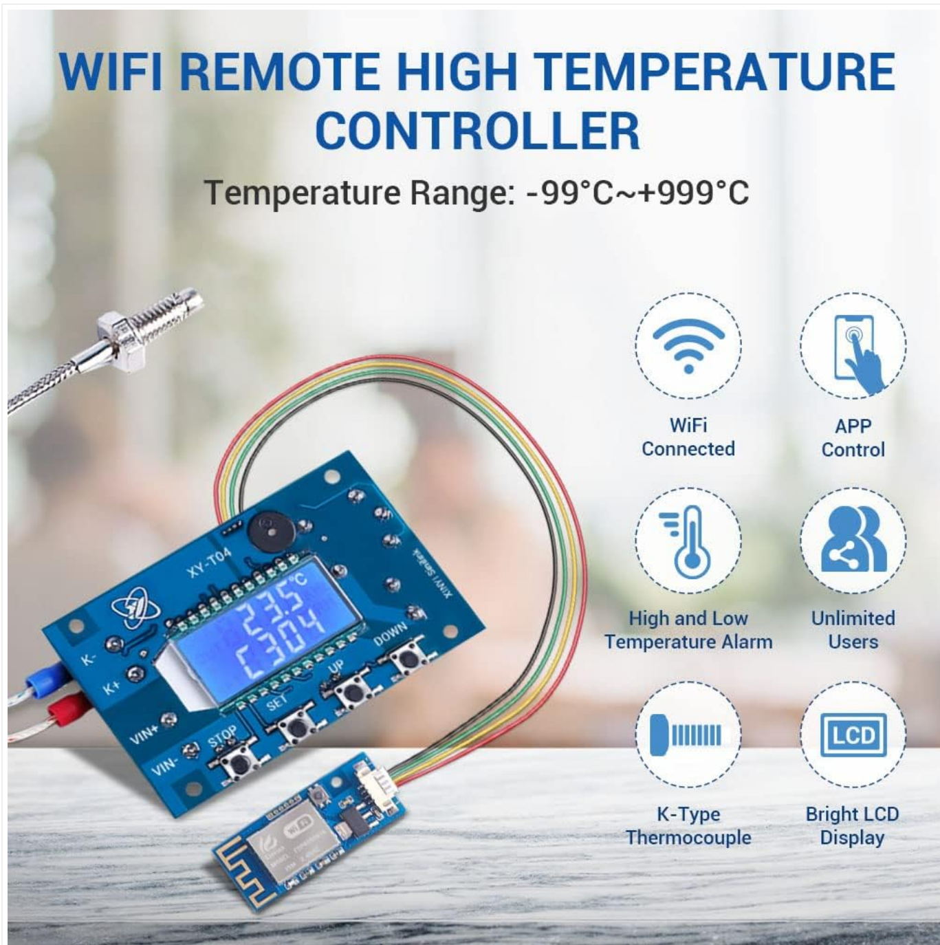
Figure 4.1: Overview of the IS GY20338 Digital Temperature Controller, showing the main board, WiFi module, and K-Type thermocouple probe.
