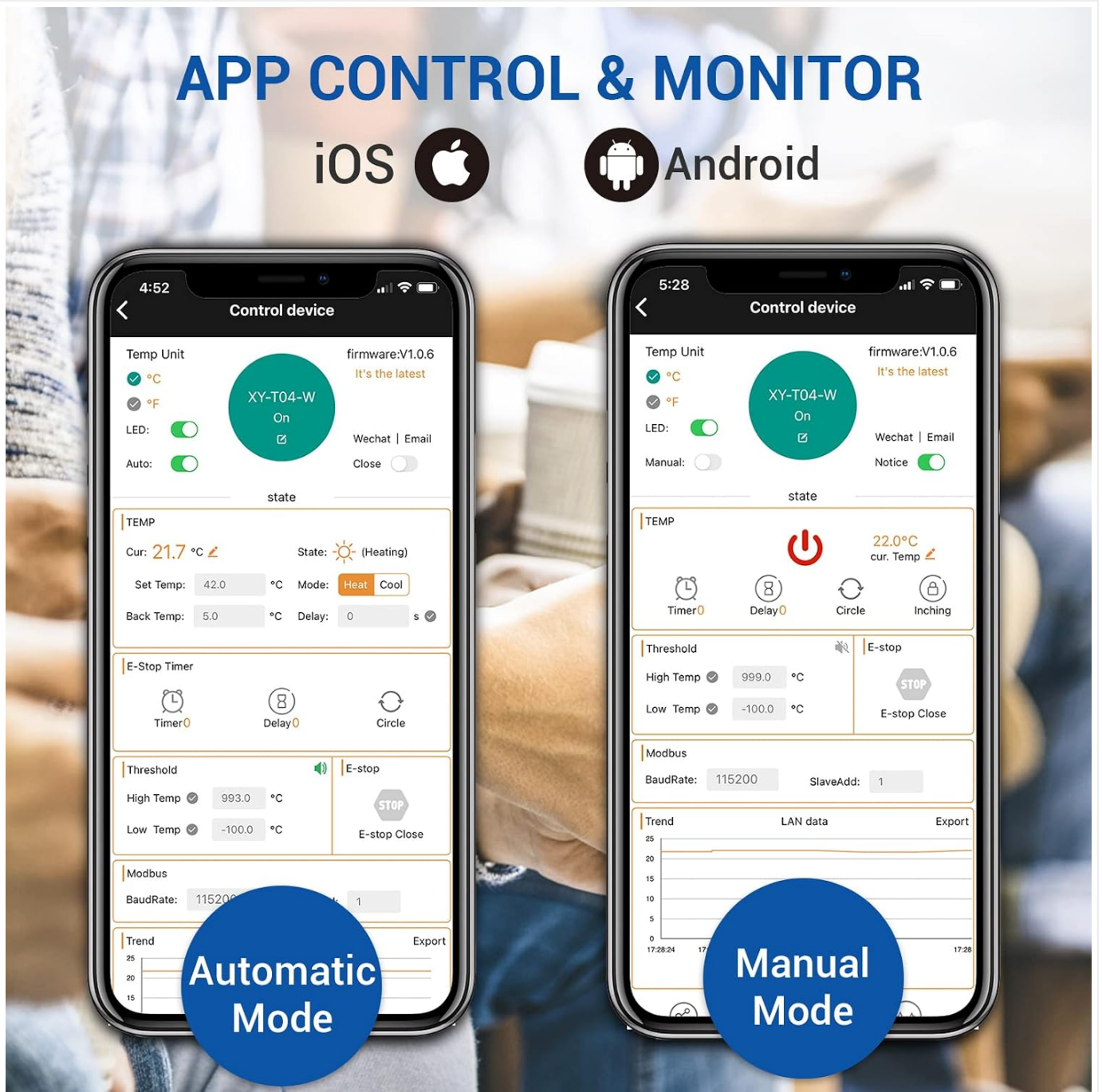
Figure 6.1: Mobile application interface for controlling the temperature module, displaying options for automatic and manual modes, temperature settings, and various functions.
