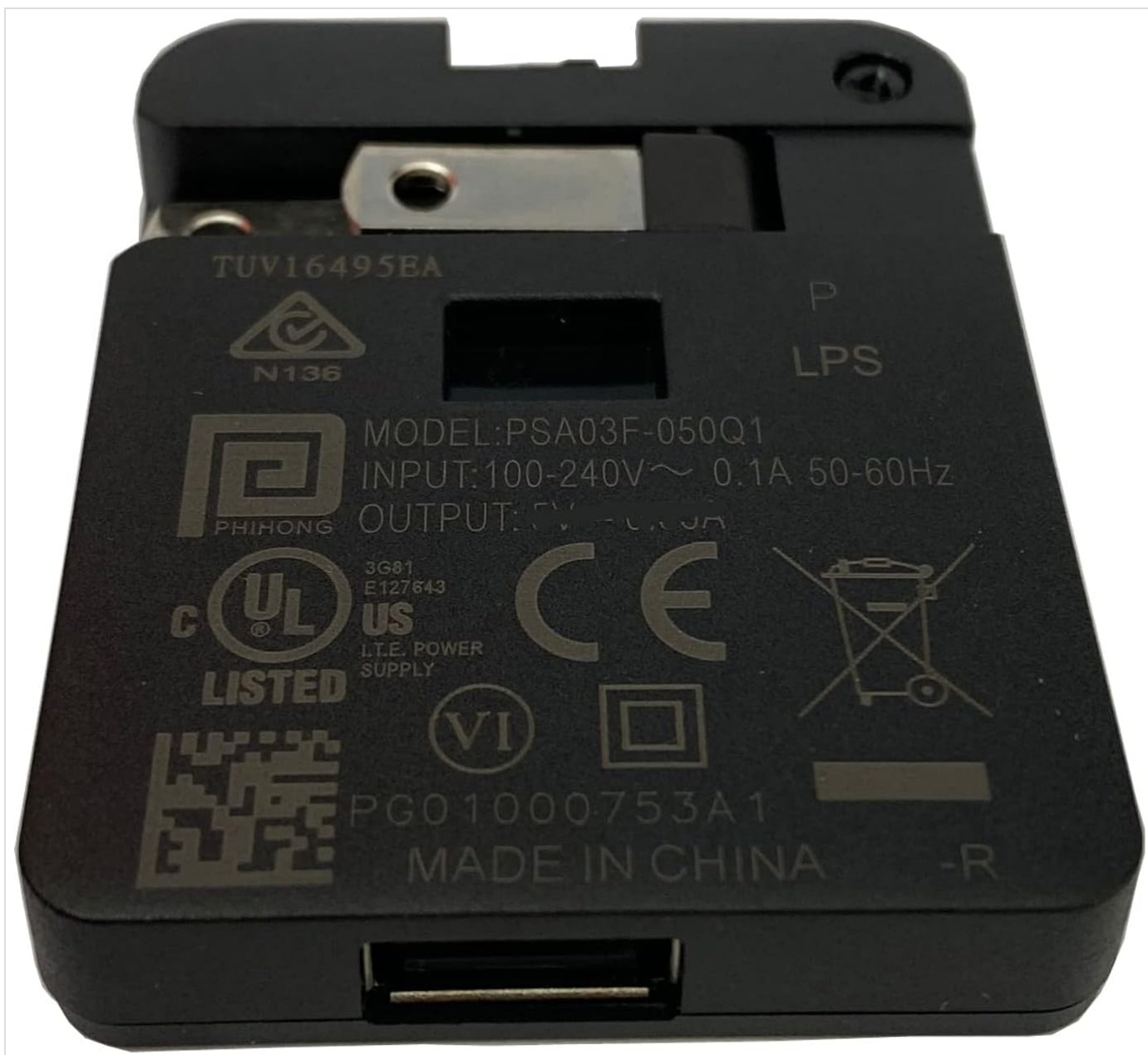
Figure 2.4: Rear view of the AC/DC Adapter. This image displays the detailed electrical specifications and certification marks printed on the back of the adapter.
