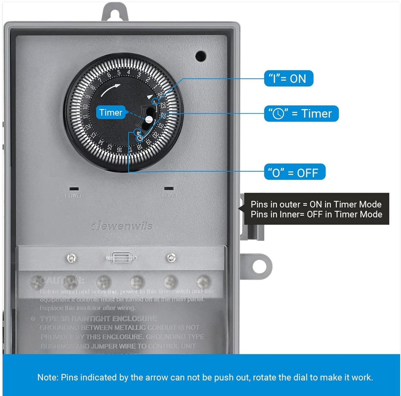
Image: A close-up of the mechanical timer dial, illustrating how to push pins out for ON periods and keep them in for OFF periods. It also shows the manual switch positions for 'I' (ON), 'Clock' (Timer), and 'O' (OFF).
