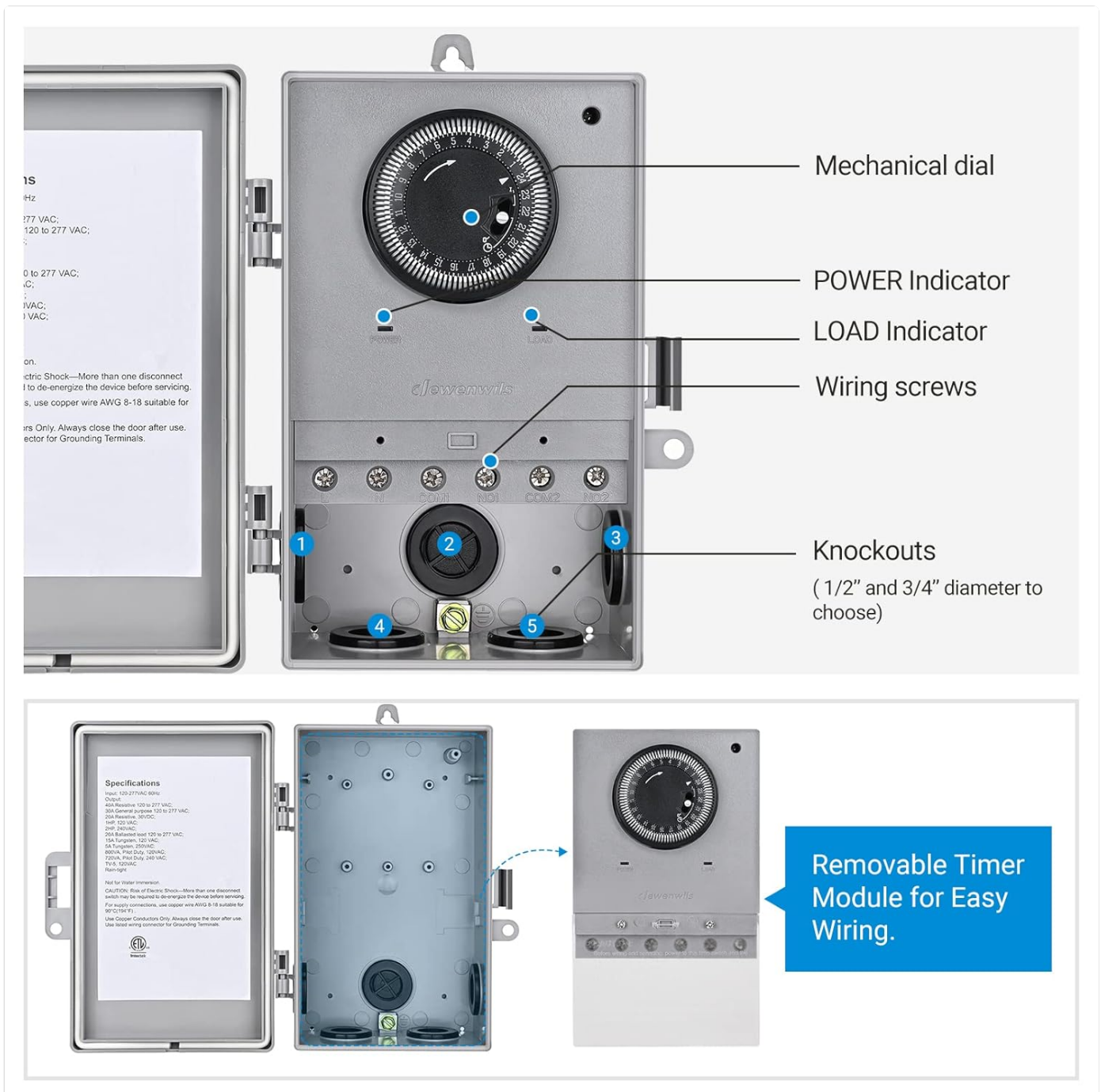
Image: Detailed diagram labeling the mechanical dial, POWER indicator, LOAD indicator, wiring screws, and knockouts (1/2" and 3/4" diameter) for conduit connections. The timer module is removable for easier wiring.
