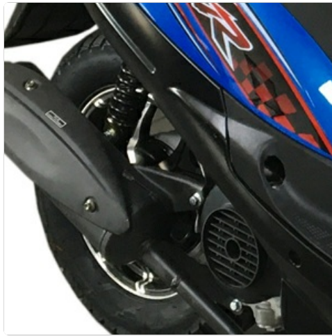
Image: Detail of the exhaust system and rear hydraulic spring suspension.
