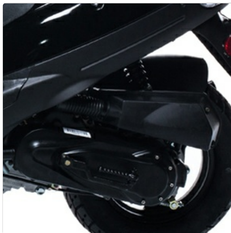
Image: View of the rear wheel and engine compartment, showing the belt-driven transmission.
