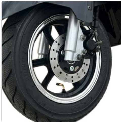
Image: Close-up of the front wheel featuring the hydraulic disc brake system.
