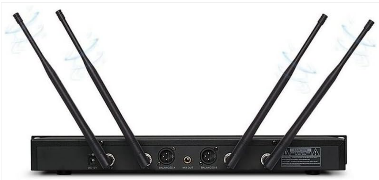
Figure 2: Rear view of the Bolymic BL-3200 receiver, highlighting the DC 12V power input, balanced XLR outputs (A and B), a mixed 1/4" output, and four antenna connections.
