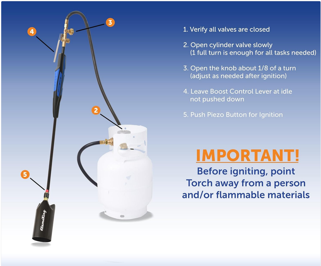
Figure 2: Step-by-step guide for connecting the torch to a propane cylinder, emphasizing the importance of verifying closed valves and proper connection.
