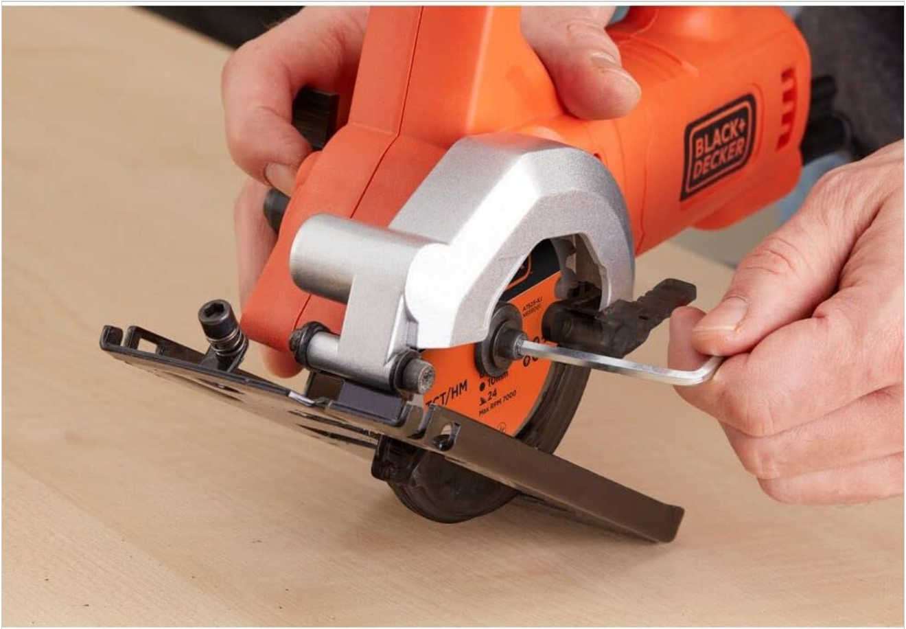
Image 4.1: A user demonstrating how to change the blade on the mini circular saw using the hex key and spindle lock. This image highlights the blade changing process.
