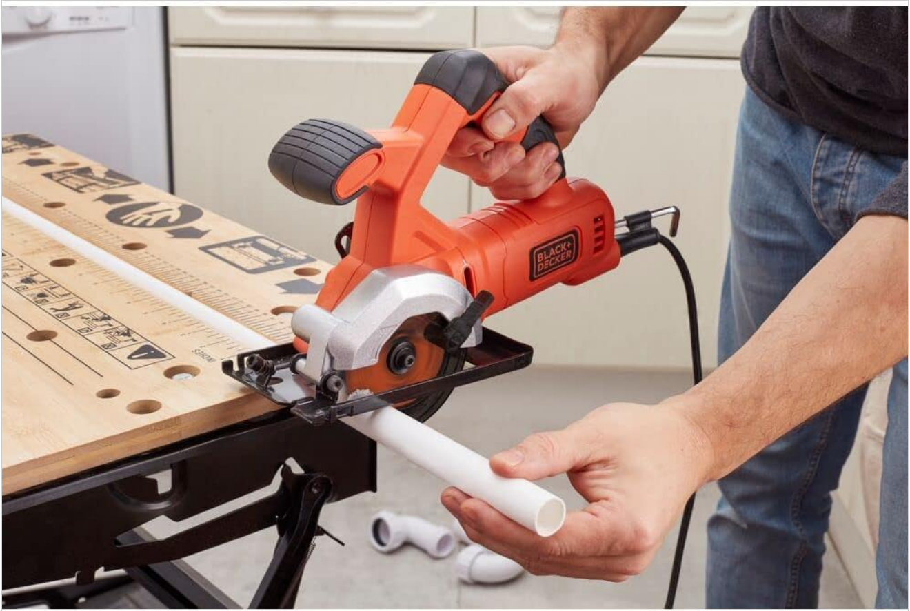
Image 5.2: A user cutting a PVC pipe using the mini circular saw, illustrating its versatility for plastic materials. This image demonstrates cutting a cylindrical object.
