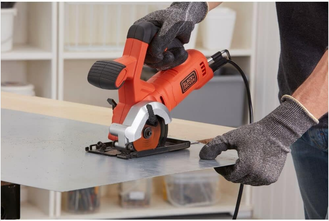
Image 5.3: A user cutting a piece of sheet metal with the mini circular saw, showcasing its capability for metalwork. This image emphasizes safety gear during metal cutting.
