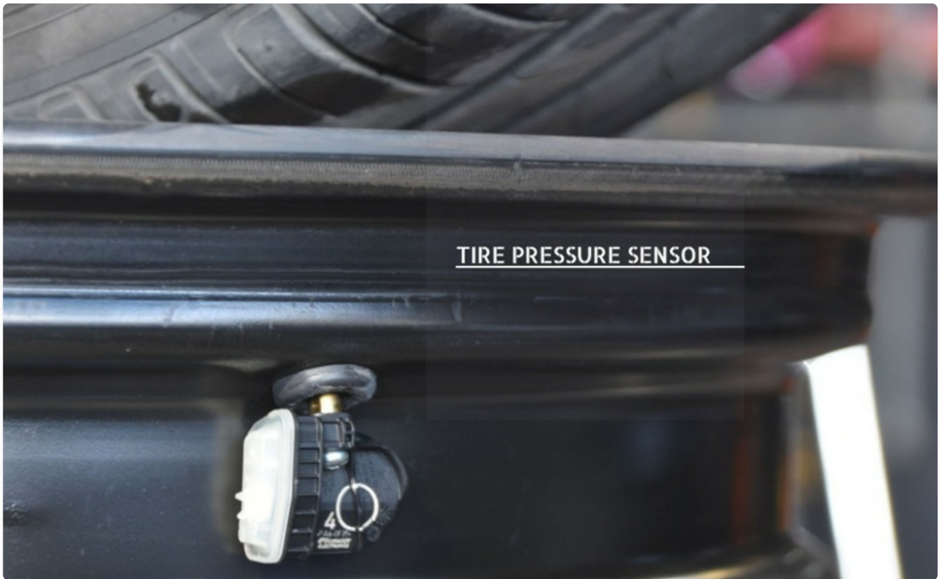
Image 1.3: A MACAX TPMS sensor correctly installed inside a vehicle's wheel rim.
