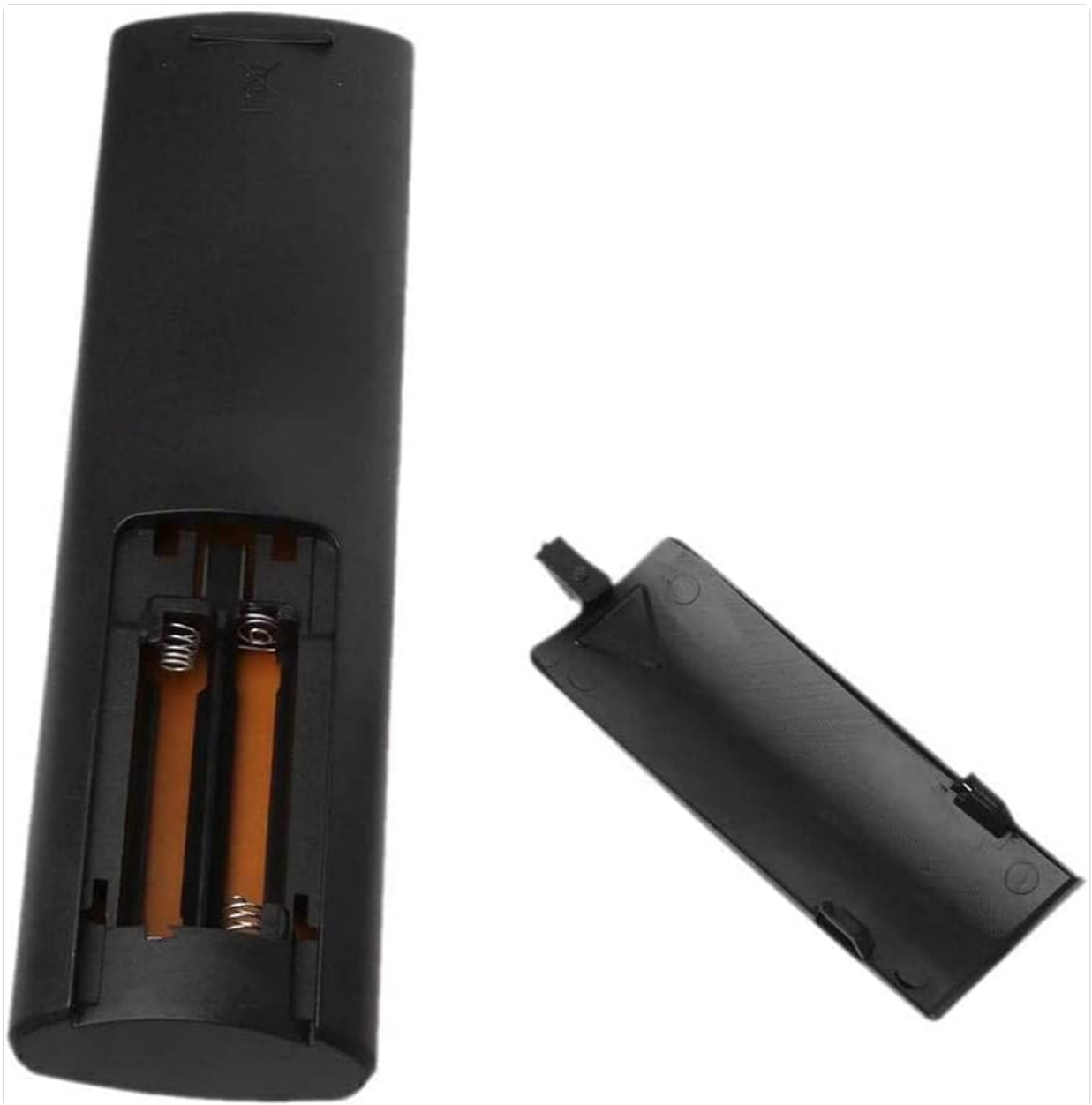
Figure 1: Battery compartment with cover removed, showing slots for two AAA batteries.
