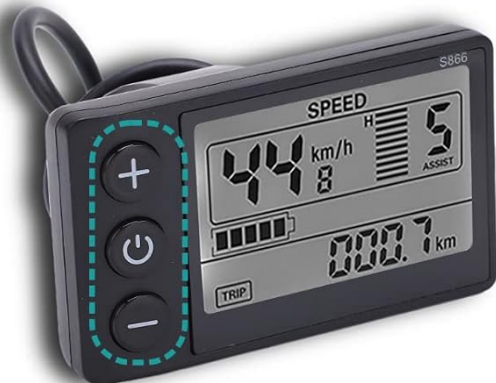
Figure 3.2: Instructions for operating the S866 LCD display, including headlight control, assist level changes, 6km/h push mode, and multi-function area navigation.
