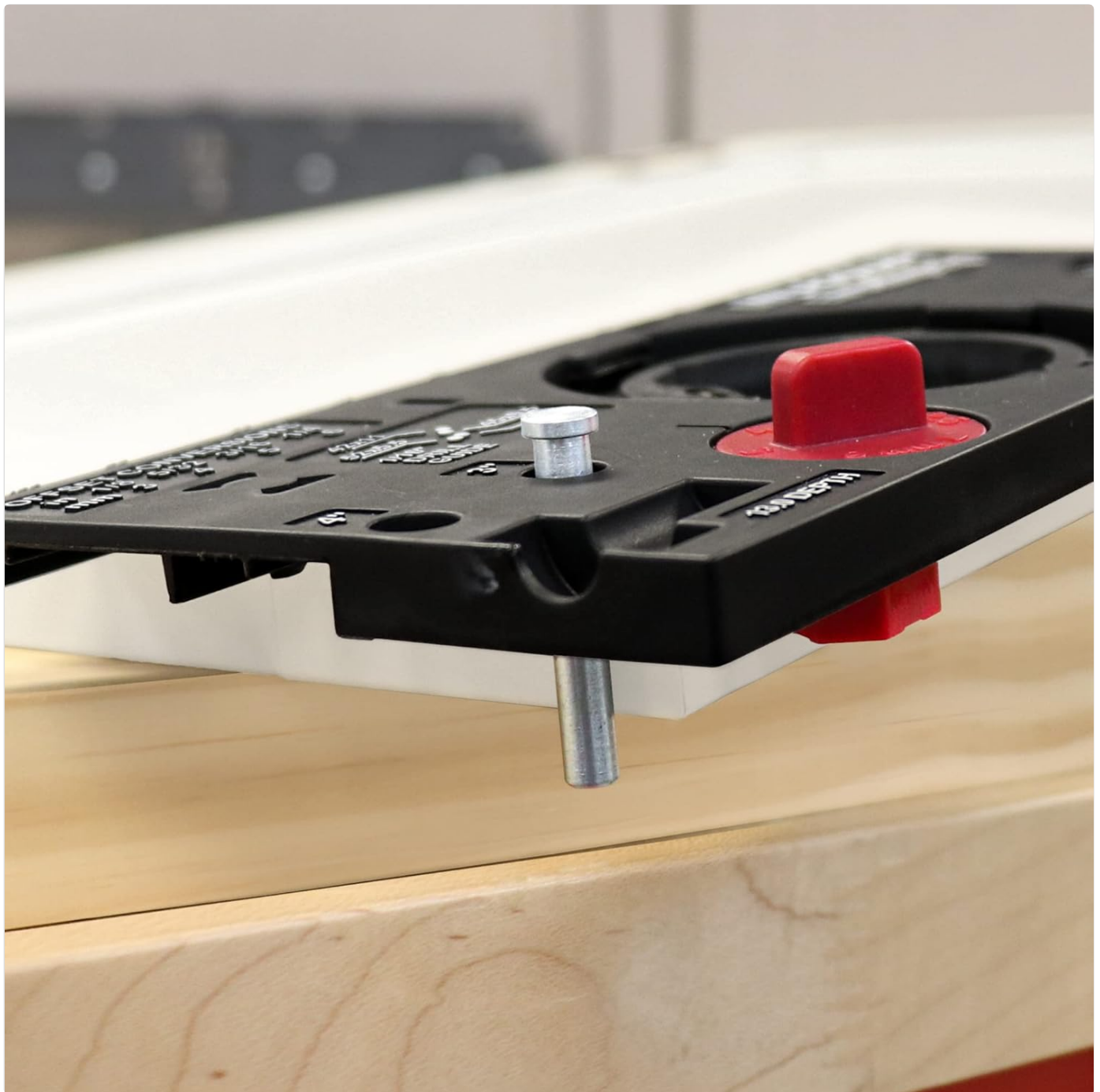
Figure 4.2: The edge locator pin ensures consistent vertical placement of hinge holes.
