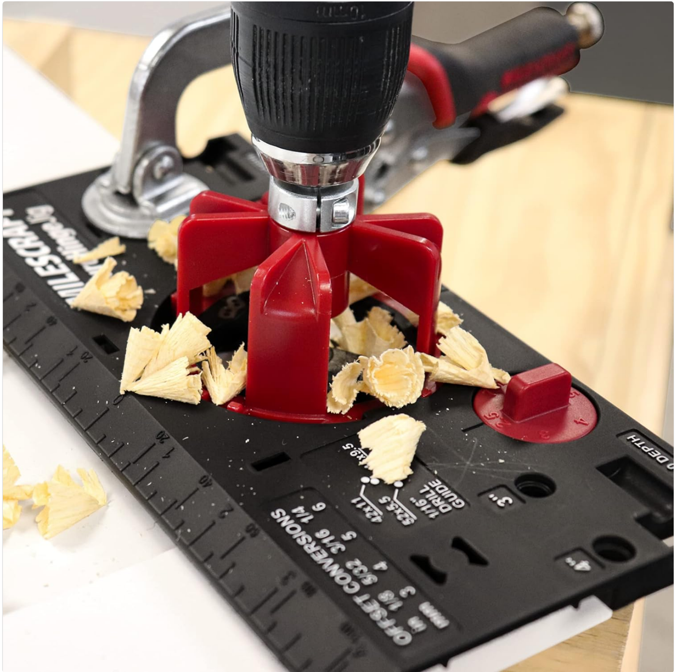
Figure 5.1: Drilling the 35mm hinge cup hole using the jig.
