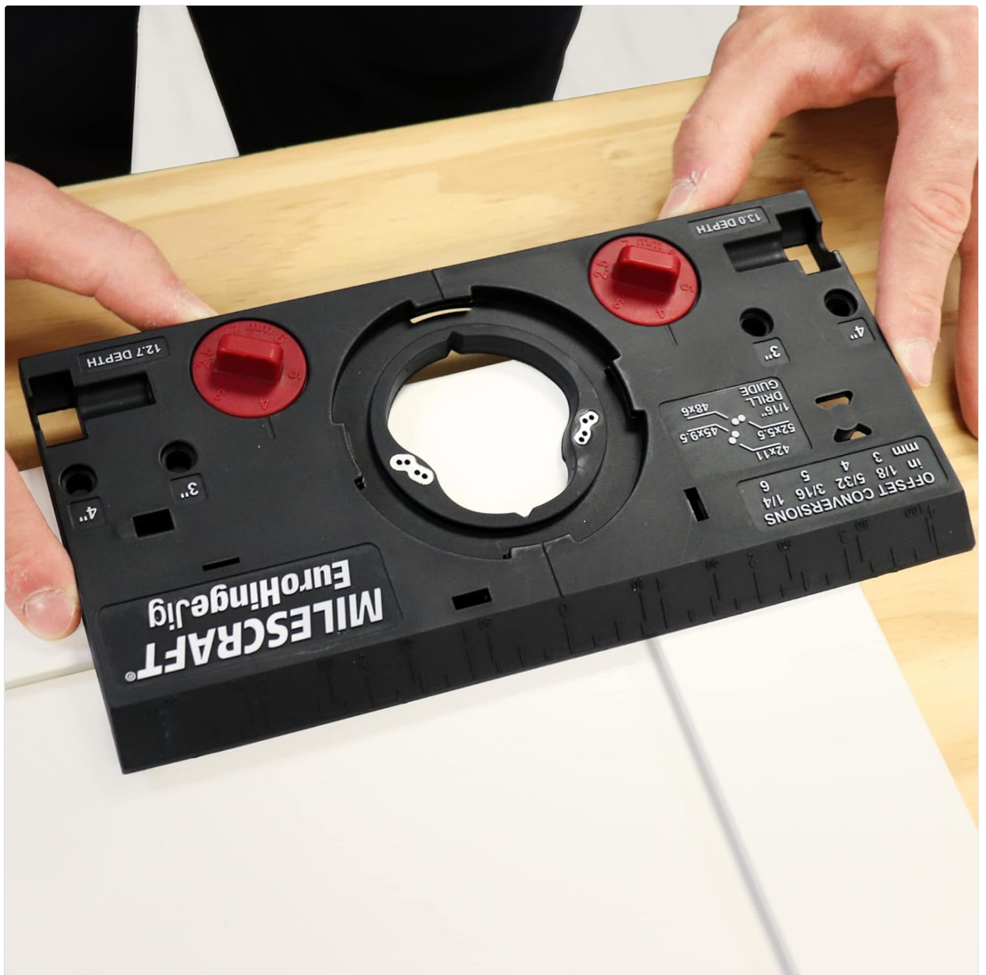
Figure 4.1: Positioning the jig on the workpiece for accurate alignment.
