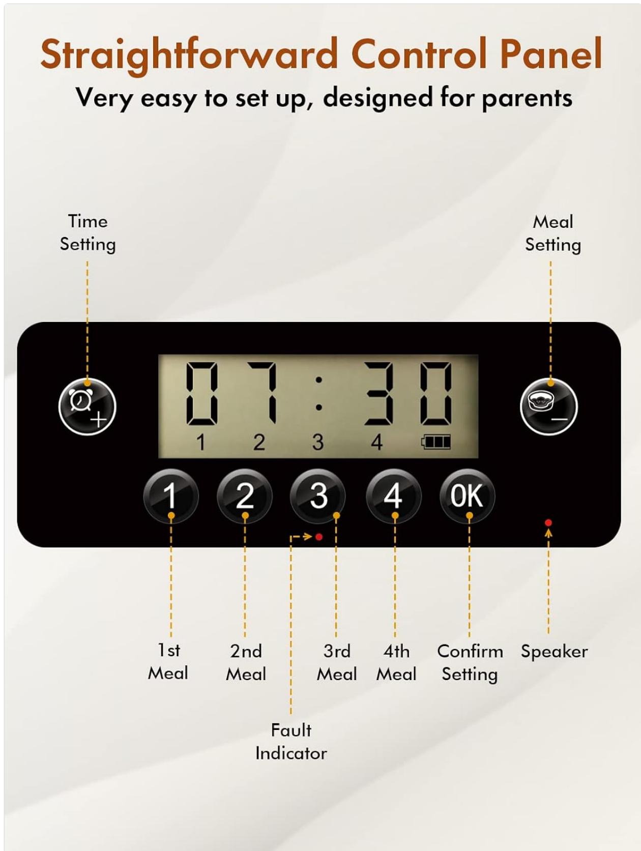
Figure 2: Detailed view of the straightforward control panel.
