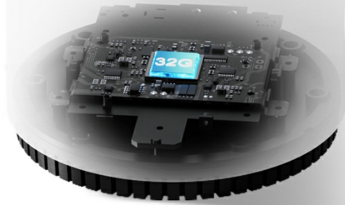
Figure 4.2: An internal view of the Homebase, emphasizing the integrated 32GB storage for secure and private local video data.
