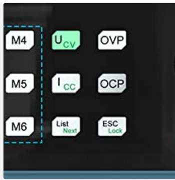
Figure 5: The memory buttons (M1-M6) allow for quick storage and recall of frequently used voltage and current settings.
