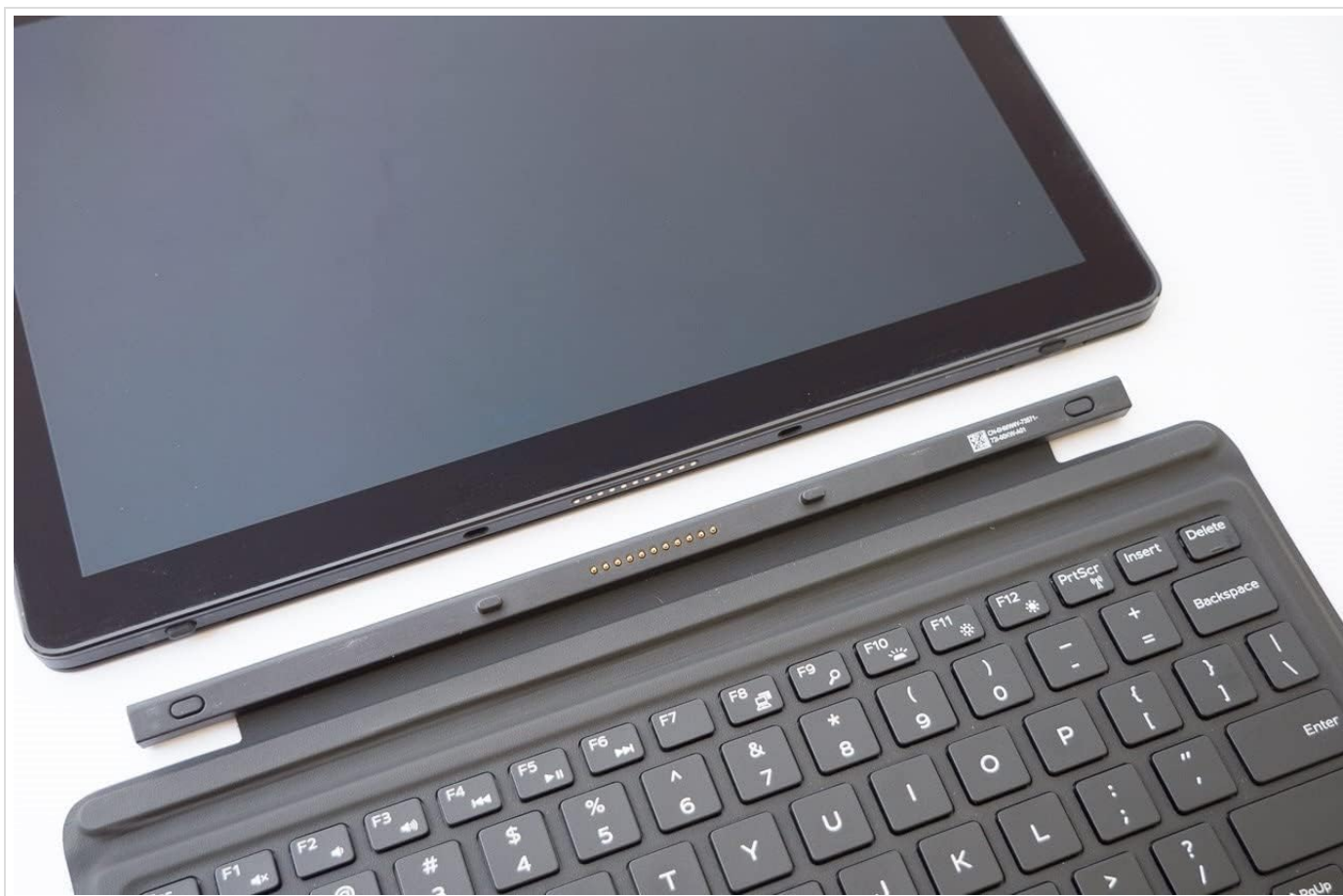
Image: A detailed view of the detachable keyboard's magnetic connector and the corresponding port on the tablet portion of the Dell Latitude 5285.
