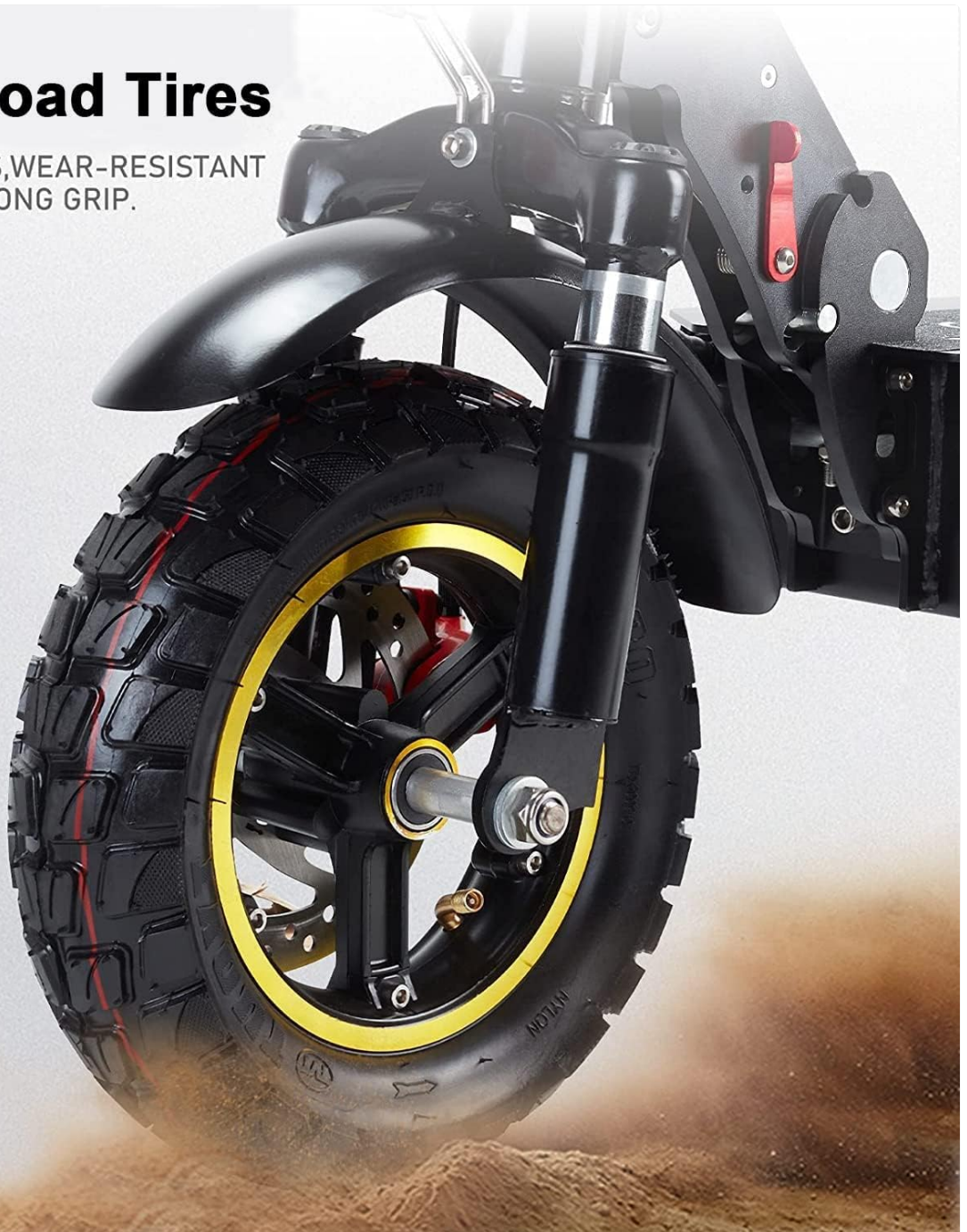
Figure 8.3: The 10-inch pneumatic off-road tires designed for various terrains.
