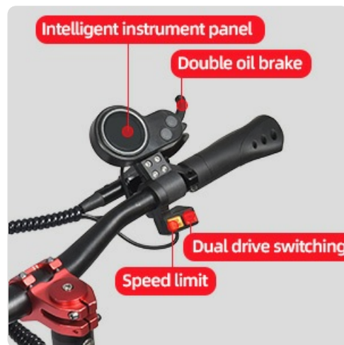
Figure 3.7: The intelligent instrument panel provides key information and controls.
