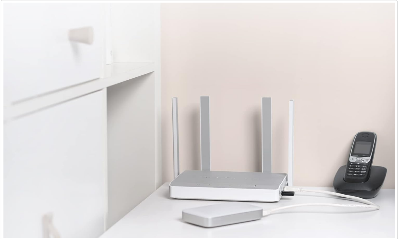
Image: The Keenetic Linéaire adapter (white rectangular device) is shown connected via a white USB cable to a Keenetic router. An analog telephone is also connected to the adapter via a telephone cable. This illustrates a typical setup configuration.
