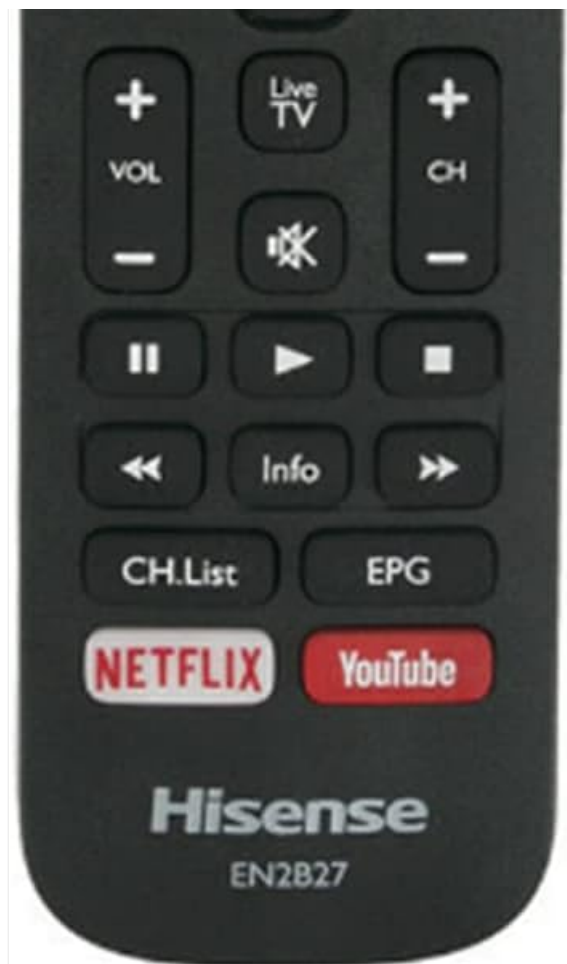
Figure 2: Front view of the EN2B27 remote control, displaying the layout of all buttons.
