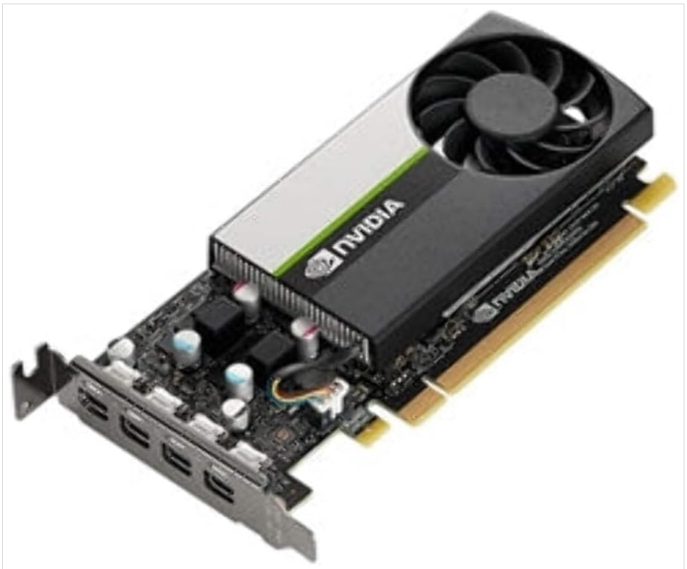
An angled view of the Acer PNY NVIDIA T1000 Graphic Card, showing the cooling fan, heatsink, and the four Mini DisplayPort outputs. This image illustrates the physical appearance of the card.
