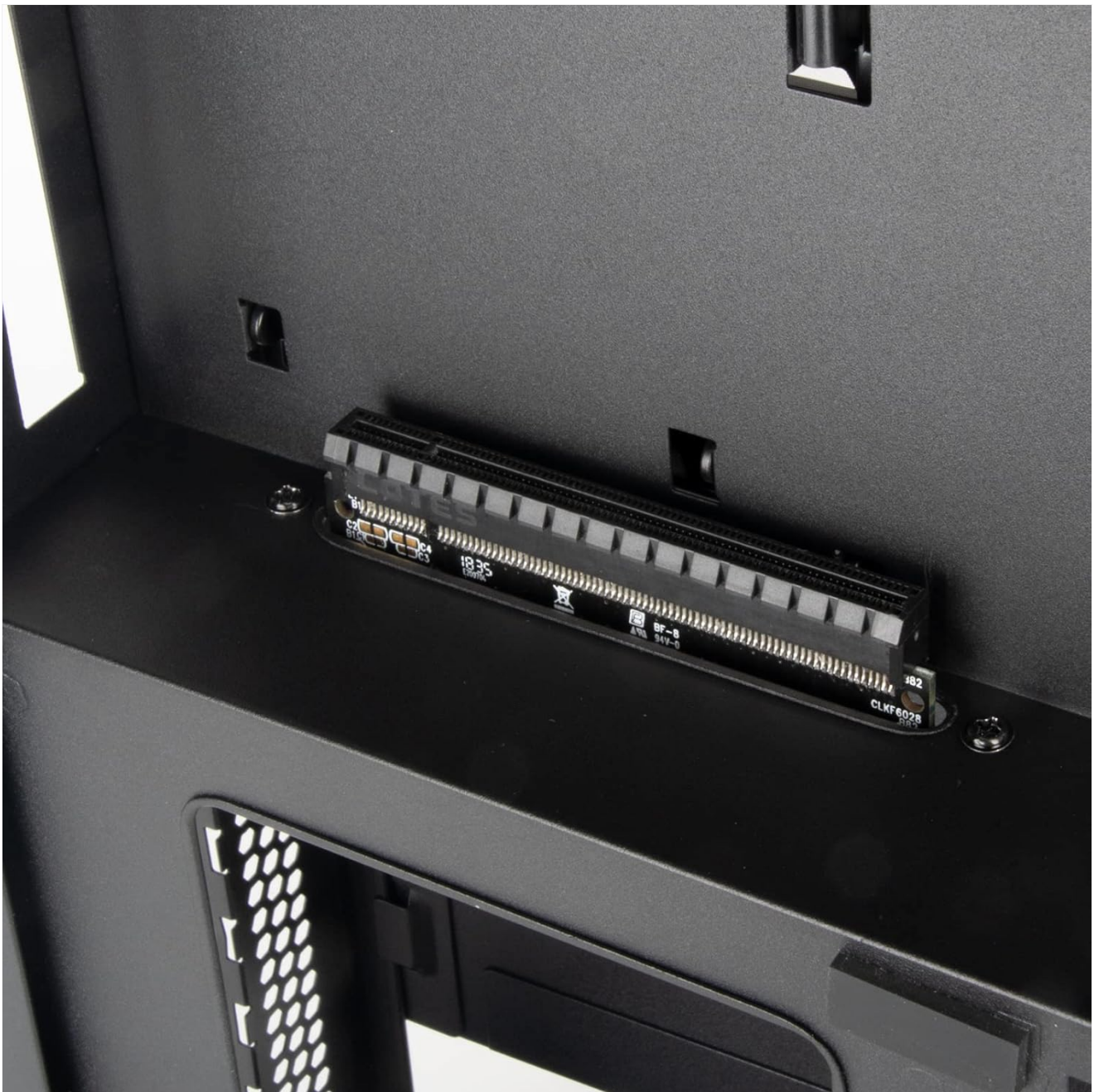
Figure 3: The SilverStone RC07 riser card installed within a compatible SilverStone chassis, showing the horizontal mounting orientation.
