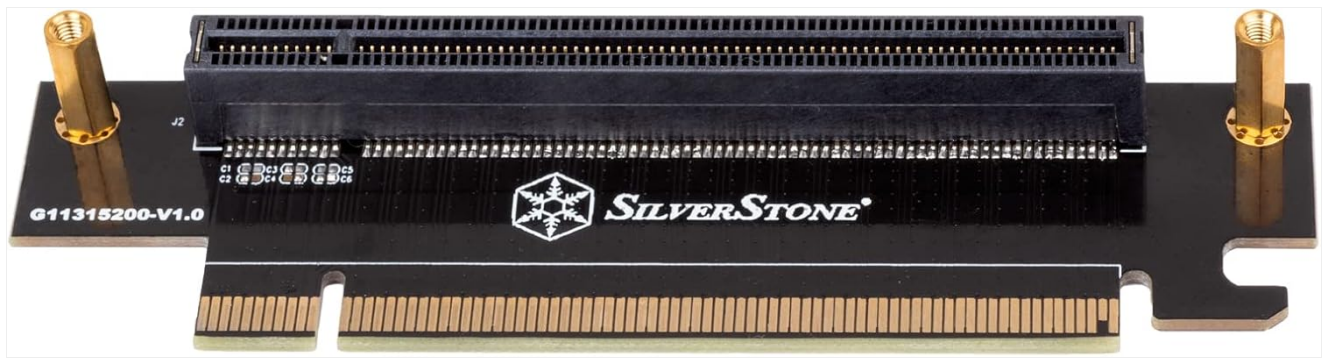
Figure 2: Angled view of the SilverStone RC07 PCI Express 4.0 x16 Riser Card, highlighting the gold-plated contacts and mounting points.
