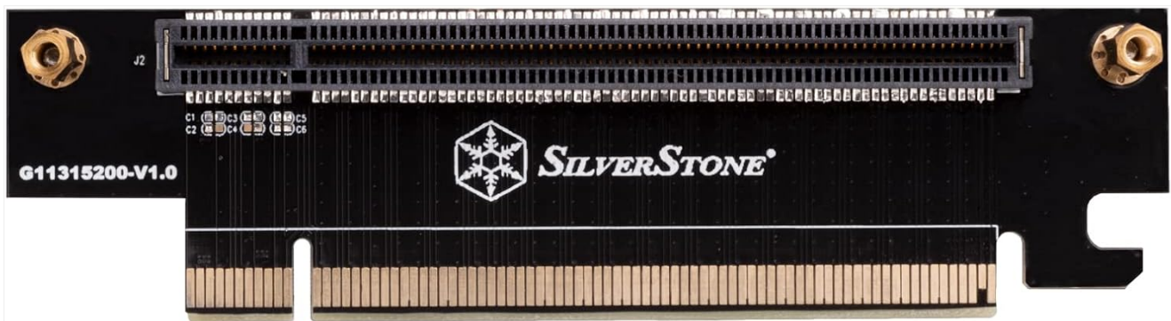
Figure 1: Top view of the SilverStone RC07 PCI Express 4.0 x16 Riser Card, showing the PCIe x16 slot and the SilverStone logo.
