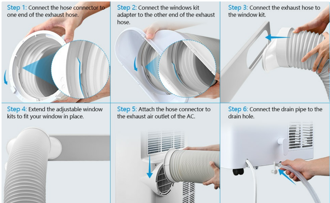
Figure 3: Installation Steps. Visual representation of connecting the exhaust hose to the window kit and the unit, and extending the window kit for proper fit.
