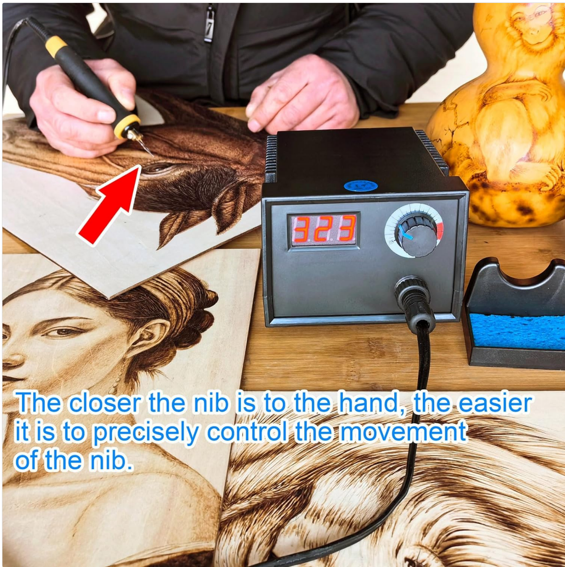
Image 5.2: Proper pen grip for enhanced control during detailed work.
