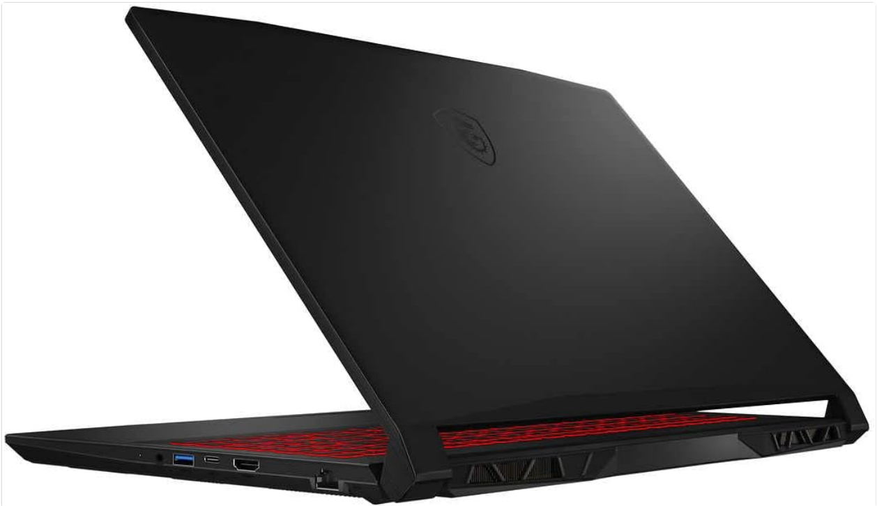
Image: Left side of the MSI Katana GF66, displaying the USB-C, USB 3.2 Gen 1 Type-A, HDMI, and power input ports.
