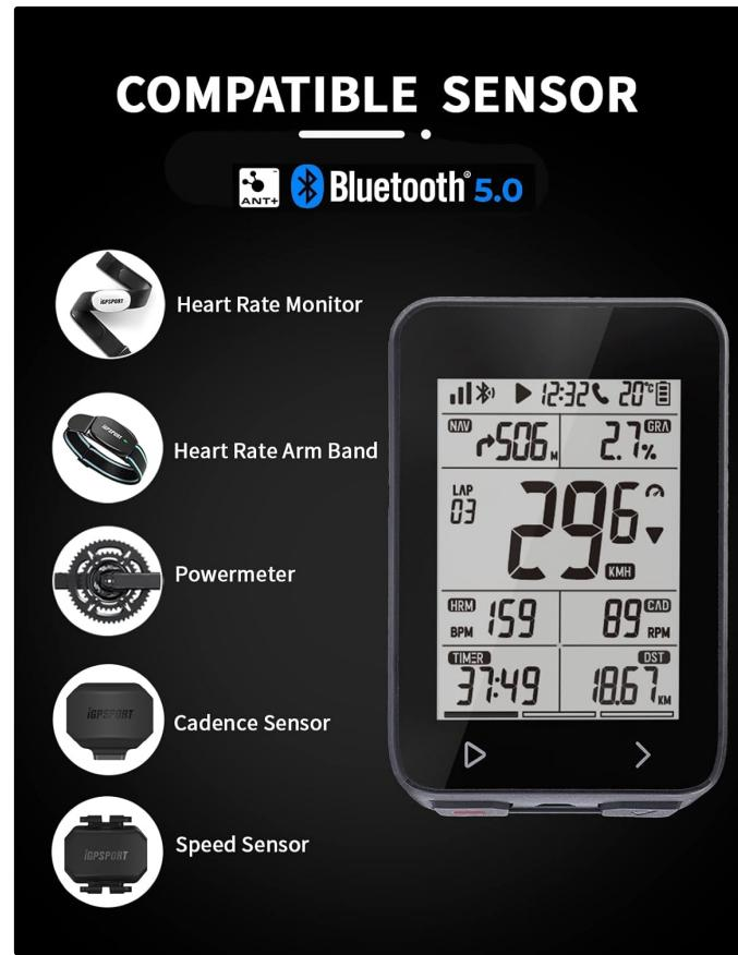
The iGS320 supports connection with multiple external sensors via Bluetooth 5.0 and ANT+ for comprehensive data collection.
