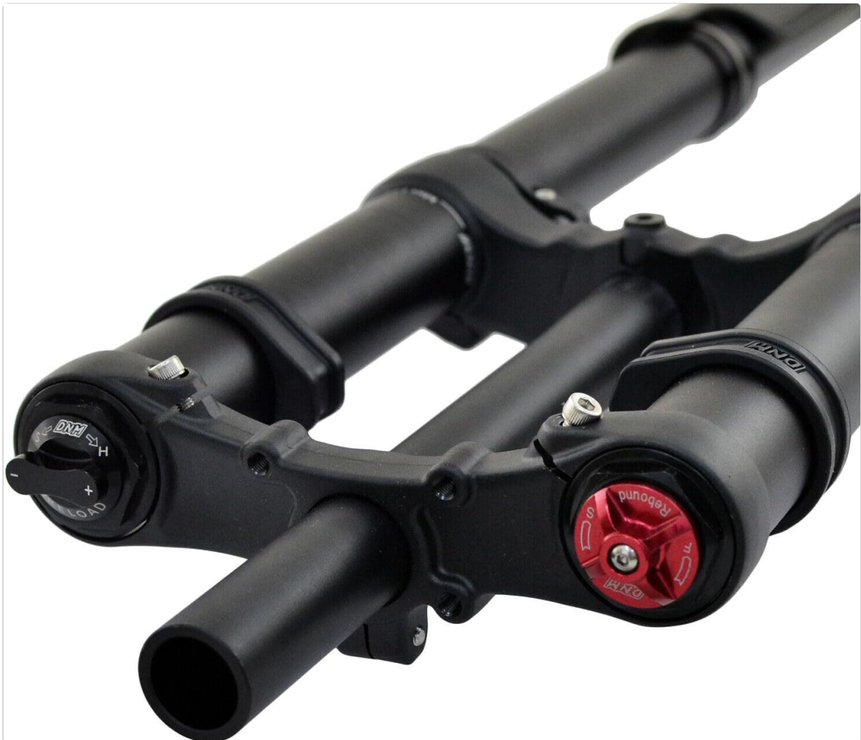
Figure 4: Close-up view of the fork's top crowns, highlighting the rebound (red) and preload adjusters.
