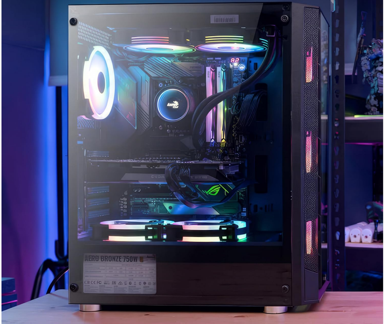
Figure 3.1: The full tempered glass side panel of the PC case, which can be removed for component installation and access.
