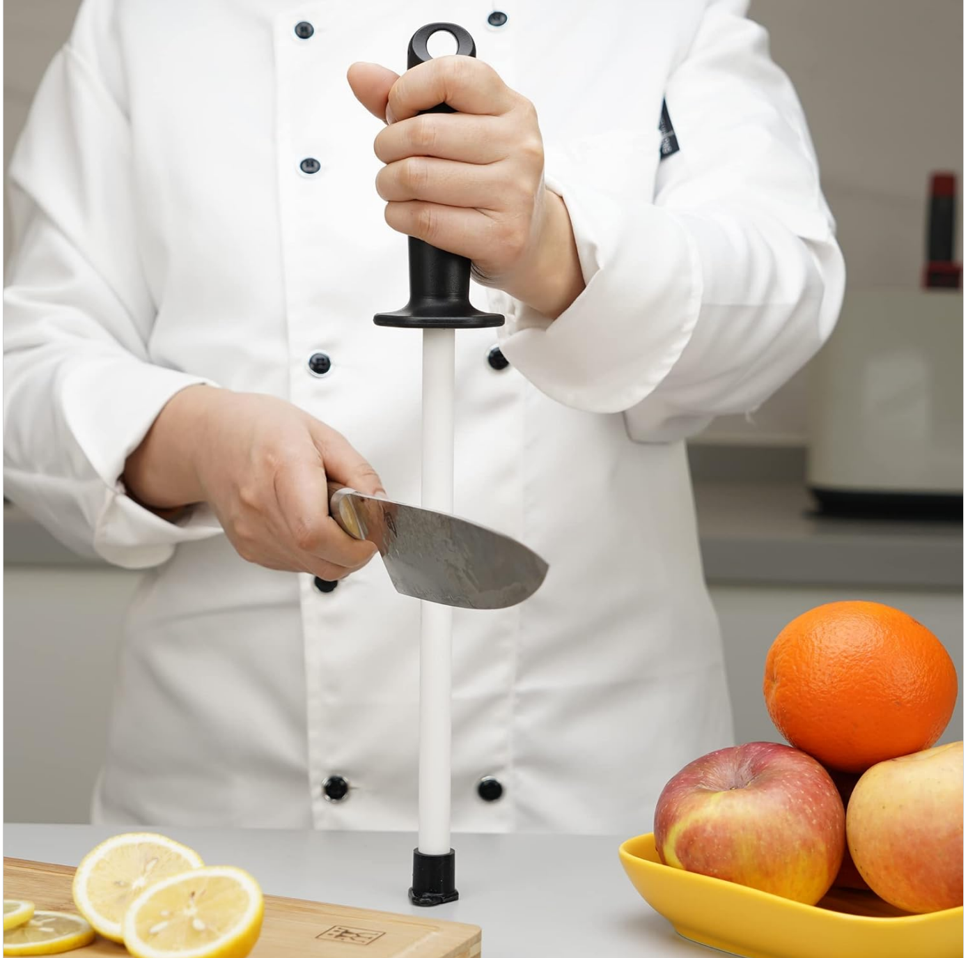
Image 4.1: A chef demonstrating the vertical sharpening technique, holding the ceramic steel upright with its tip on a surface and drawing the knife blade down.
