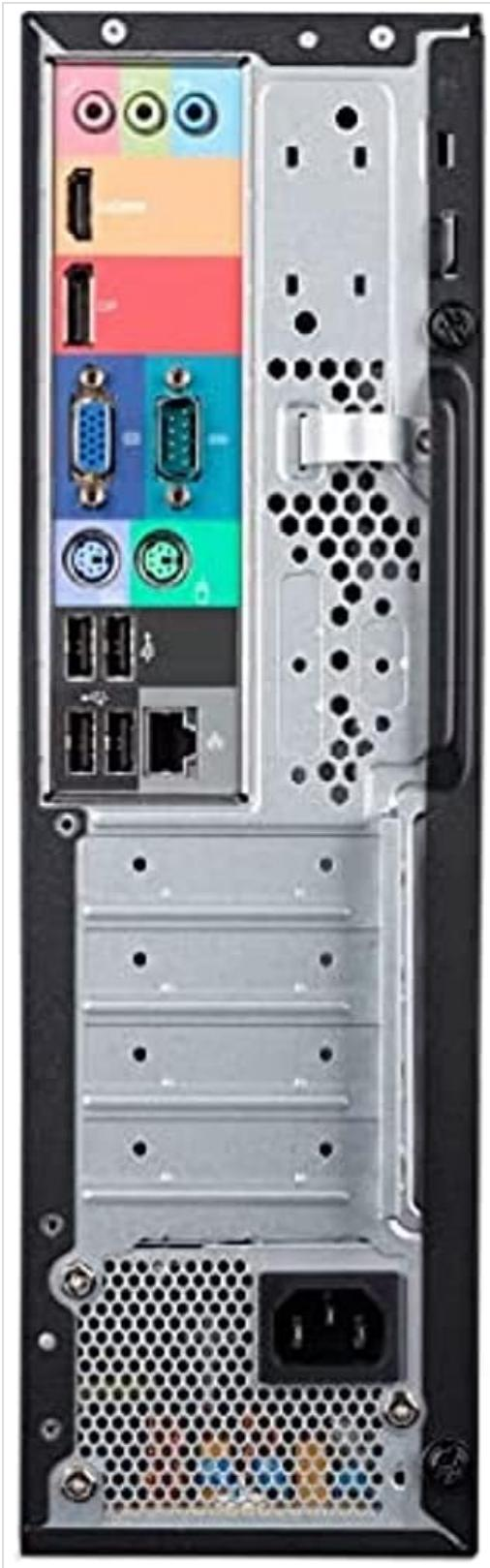
This image shows the rear panel of the Acer Veriton X4680G, detailing the various input/output ports. These include multiple USB ports, Ethernet port, audio jacks, video output ports (VGA, DisplayPort), and the power input connector. Expansion slots are also visible.
