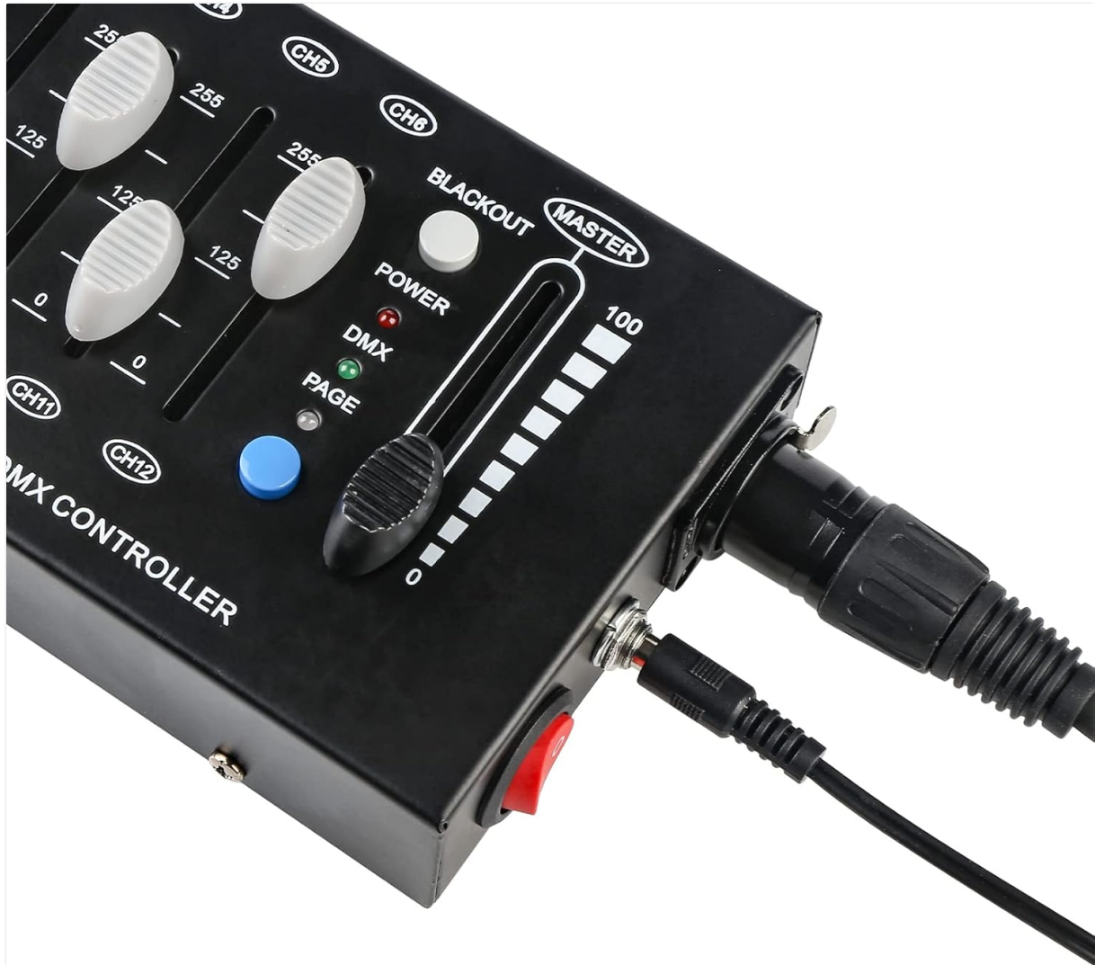
Image: The DMX output (XLR 3-pin) and DC power input ports with connected cables.
